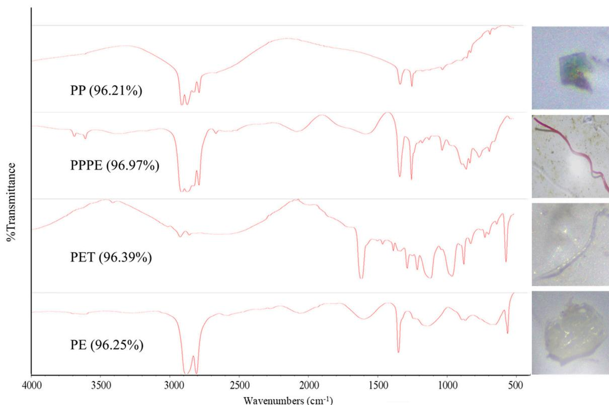
**Figure 2.** Typical  $\mu$ -FTIR spectra of microplastics detected in multiple-used zones in Eastern Guangdong, the South China Sea; PP: poly(propylene); PPPE: polypropylene-polyethylene copolymer; PET: polyethylene terephthalate; PE: polyethylene; percentage in the bracket: matching degree with the standard.
