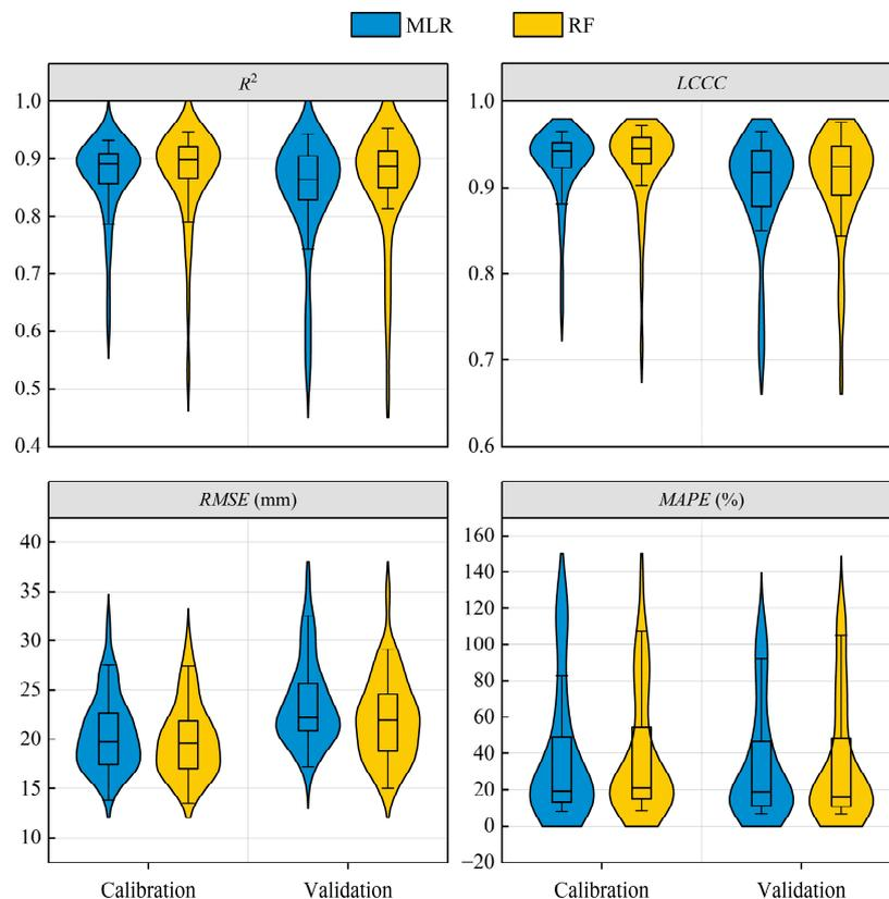
Figure 6. Results of  $R^2$ , LCCC, RMSE, and MAPE to show performance of MLR- and RF-based models for site-specific  $D$  in northwestern China during the calibration and validation processes. The horizontal line inside the box indicates the median. The box boundary indicates the 25th and 75th percentiles, and the whiskers below and above the box indicate the 10th and 90th percentiles.
