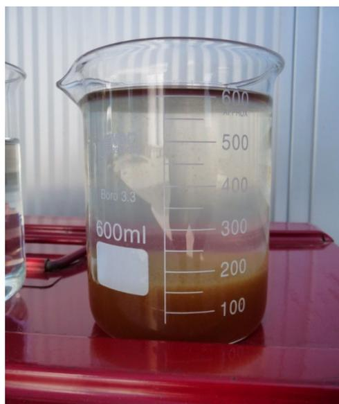
**Figure 4.** Reject water after 30 min sedimentation.
