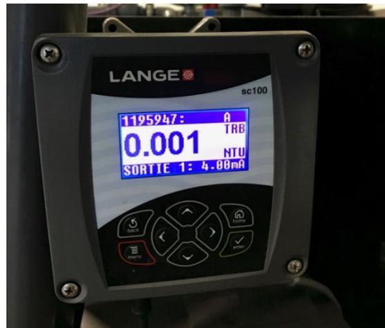
**Figure 2.** Typical turbidity reading during the filtration period.
