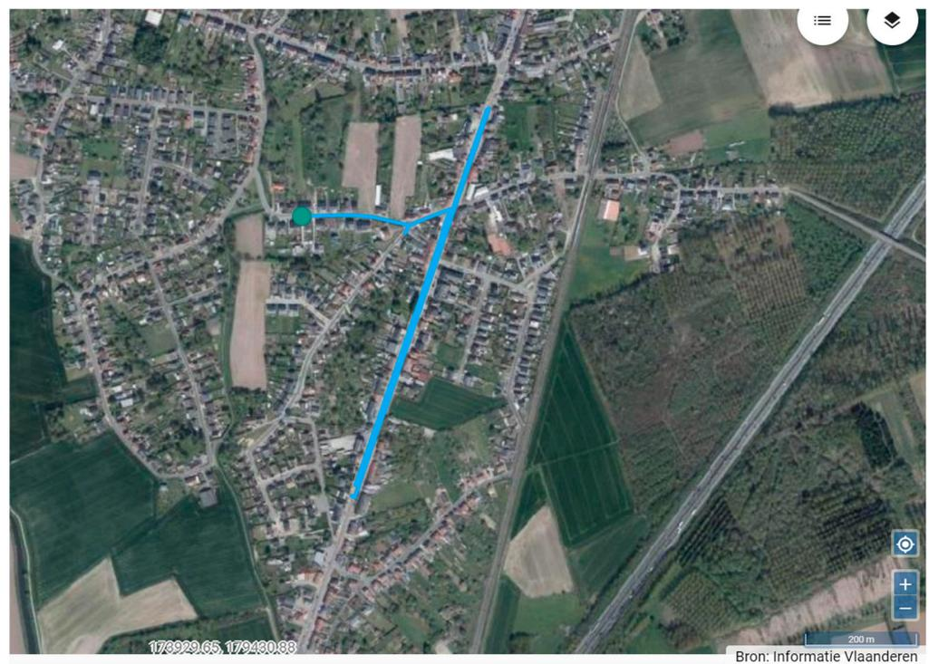
**Figure A2.** Overview of the catchment in Wilsele. The green dot shows the inspection well where the samples were taken. The blue area is connected to the inspection well.
