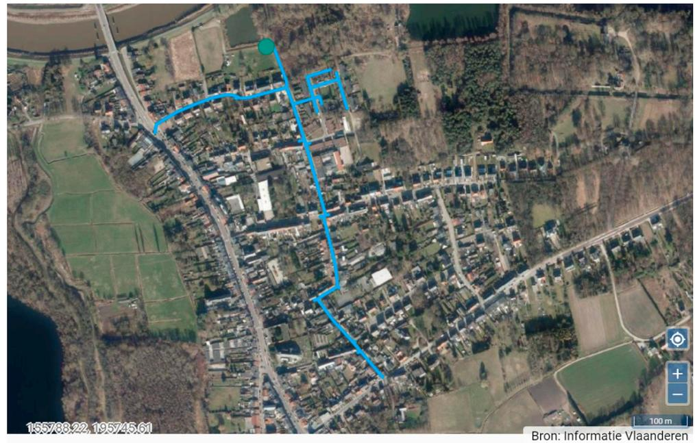
**Figure A1.** Overview of the catchment in Wilsele. The green dot shows the inspection well where the samples were taken. The blue area is connected to this inspection well.
