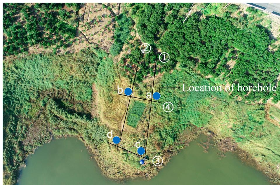
Figure 14. Layout of the high-density electrical survey line of the Baijiabao landslide.
