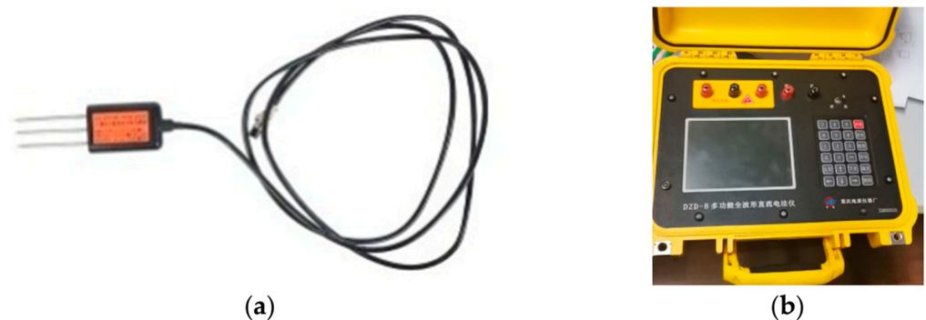
Figure 8. Monitoring instrument: (a) LD-EC soil moisture sensor, (b) DZD-8 multifunctional full-waveform DC electrostatic instrument.
