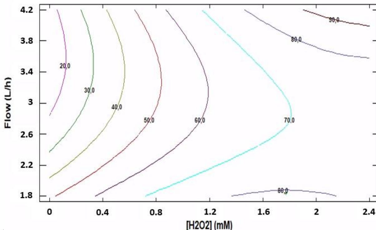
**Figure 6.** Surface response obtained for the removal of acetaminophen in continuous mode. The % of removal at the exit of the reactor is plotted vs. the concentration of  $\text{H}_2\text{O}_2$  and the flow rate.
