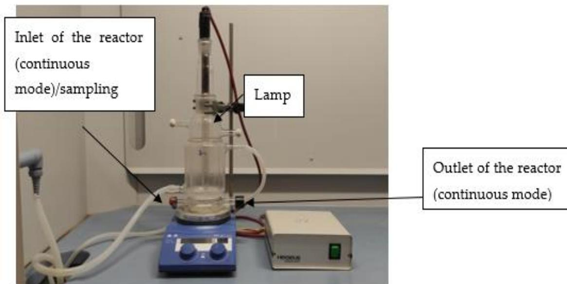
**Figure 1.** Experimental set-up employed in this work.
