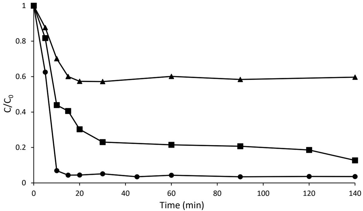
**Figure 4.** Plot of the relative concentration of acetaminophen at the outlet of the reactor when operated in the continuous mode under different conditions: UVC (▲), UVC + H<sub>2</sub>O<sub>2</sub> (21 mM) (■) and UVC + H<sub>2</sub>O<sub>2</sub> (21 mM) + bubbling air (●).
