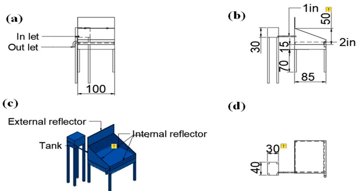
**Figure 2.** AutoCAD designing of fabricated solar still (a–d).
