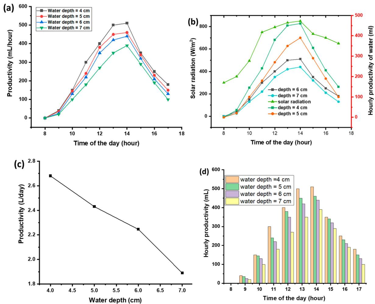
**Figure 5.** Productivity varies with water depth and time. Productivity with daytime (a), solar radiation with daytime (b), productivity per day with water depth (c), Bar diagram of hourly productivity at different water depths (d).
