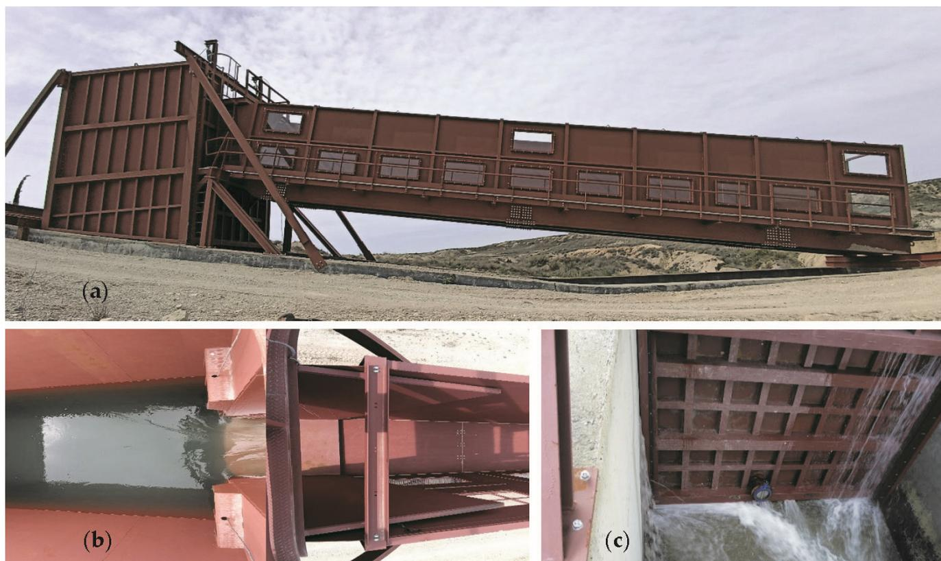
**Figure 5.** (a) General view of the supply tower and the test chute before being lowered to the bottom of the auxiliary channel (b) Photographic montage of the water inside the supply tower (left) exiting towards the test chute (right). (c) Wall gate of the supply tower and 250 mm diameter butterfly valve to facilitate its operation by emptying the water retained upstream.
