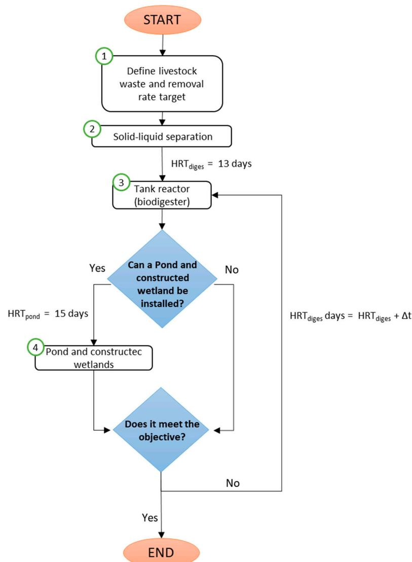
Figure 3. Flow diagram tool for NTSW design.
