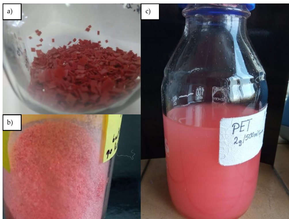
Figure 1. Prepared samples of microplastics. (a) cut plastic ketchup bottle made of PET; (b) milled and sieved microparticles; (c) stock suspension of the microplastics.
