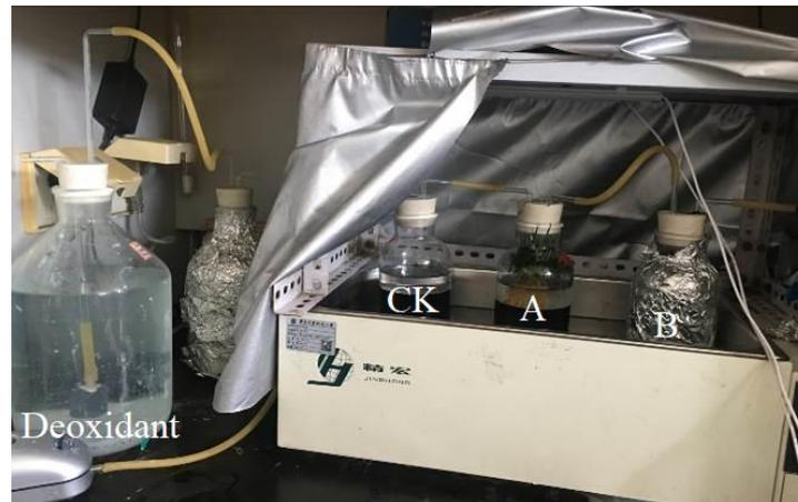
**Figure 1.** System for measuring radial oxygen loss measurement.
