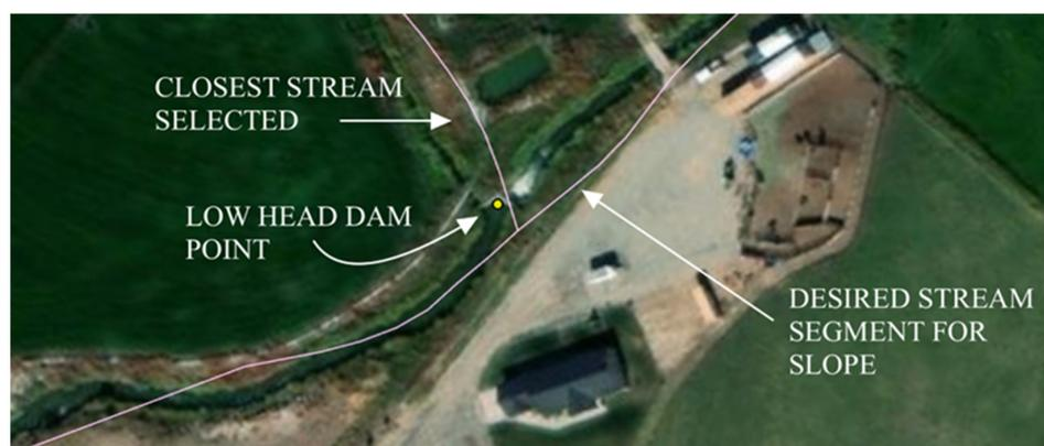
**Figure 6.** Example of a stream selection error for a low head dam with no fatalities in Idaho.
