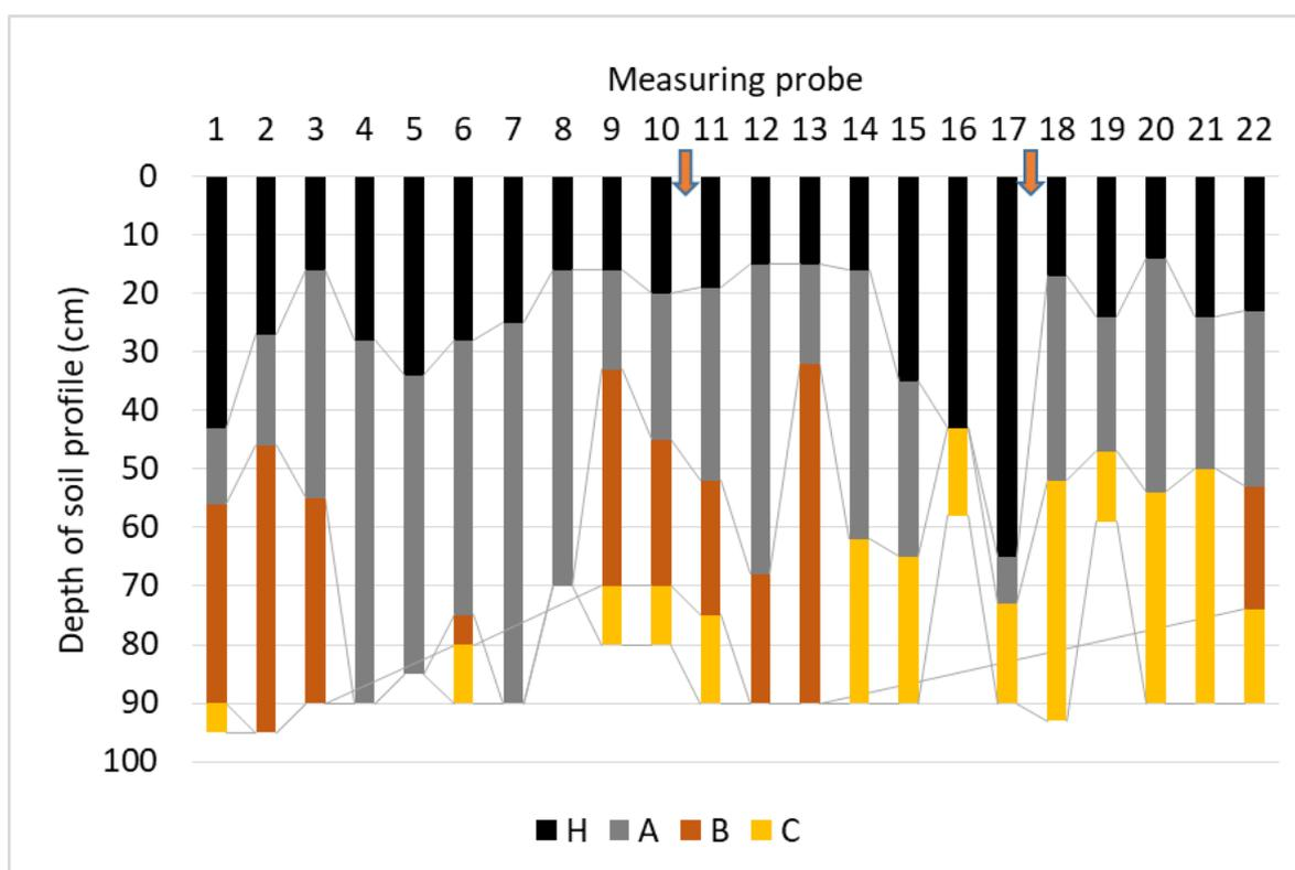
**Figure 3.** Soil profile horizons of the measuring probes (1 to 22; from lower to higher altitudes, see Figure 1) in the year of installation (1992). H—humified organic layer, A, B, C—mineral horizons. Arrows depict placement of the drainage ditches in 1995.
