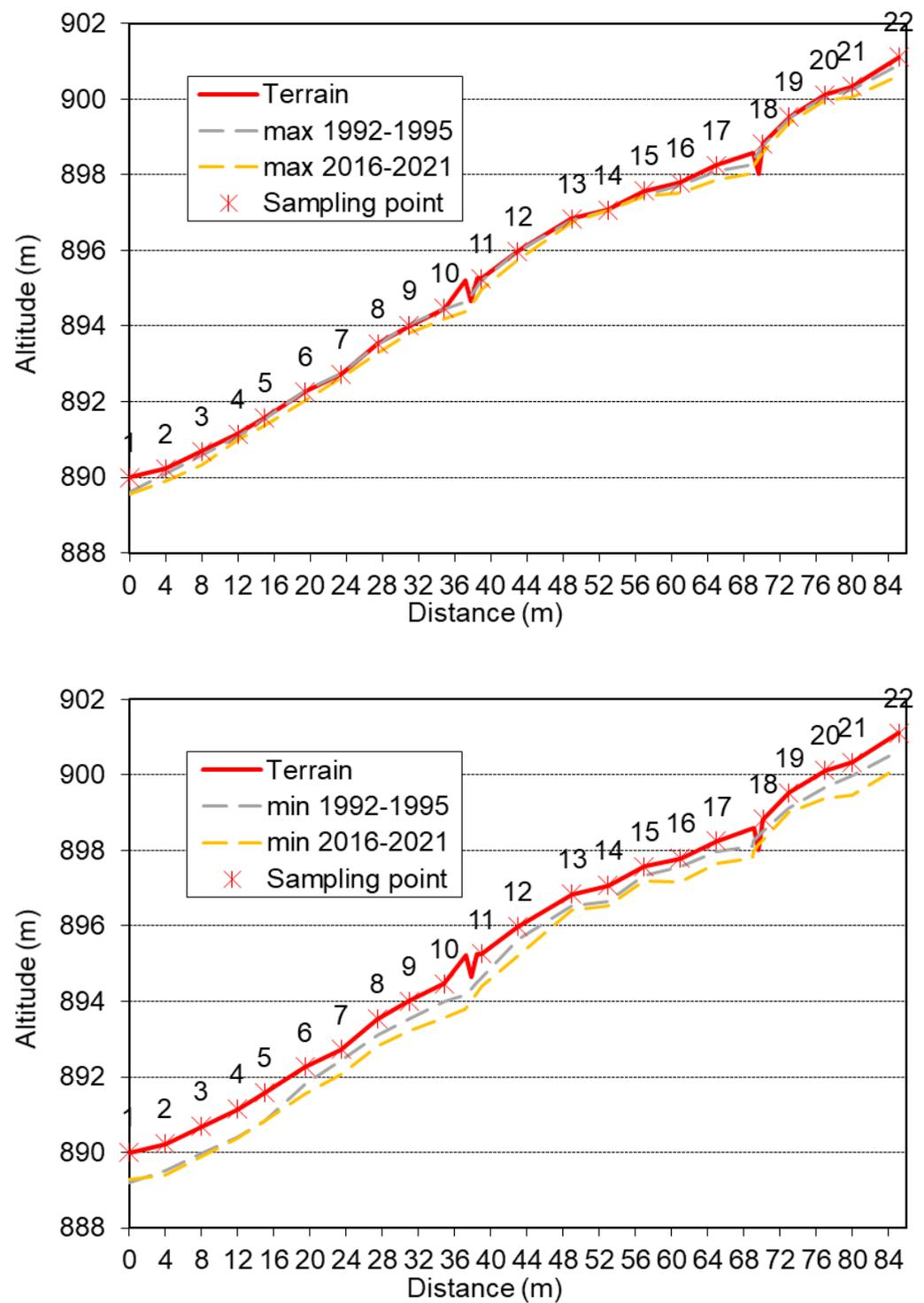
**Figure 11.** Slope of the experimental transect area and the average minimum (**above**) and maximum (**below**) GWTs during the vegetation periods of 1992–1995 (a mostly deforested, calibration period before the drainage system was constructed) and 2016–2021 (the last period, forest cover restored). The numbers represent the position of the measuring probes.
