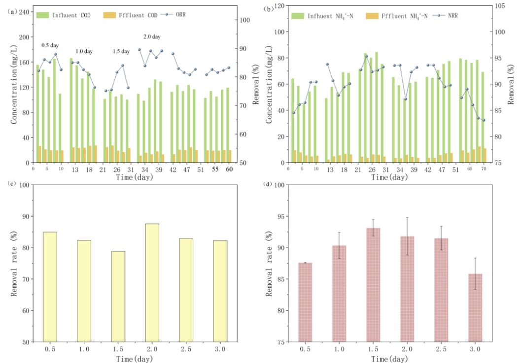
**Figure 2.** Removal of COD and  $\text{NH}_4^+\text{-N}$  under different intermittent aeration times: (a) removal of COD under the influence of intermittent aeration, (b) removal of  $\text{NH}_4^+\text{-N}$ , (c) comparison of COD removal rates under 6 intermittent aeration conditions, (d) comparison of  $\text{NH}_4^+\text{-N}$  removal rates under 6 intermittent aeration conditions.
