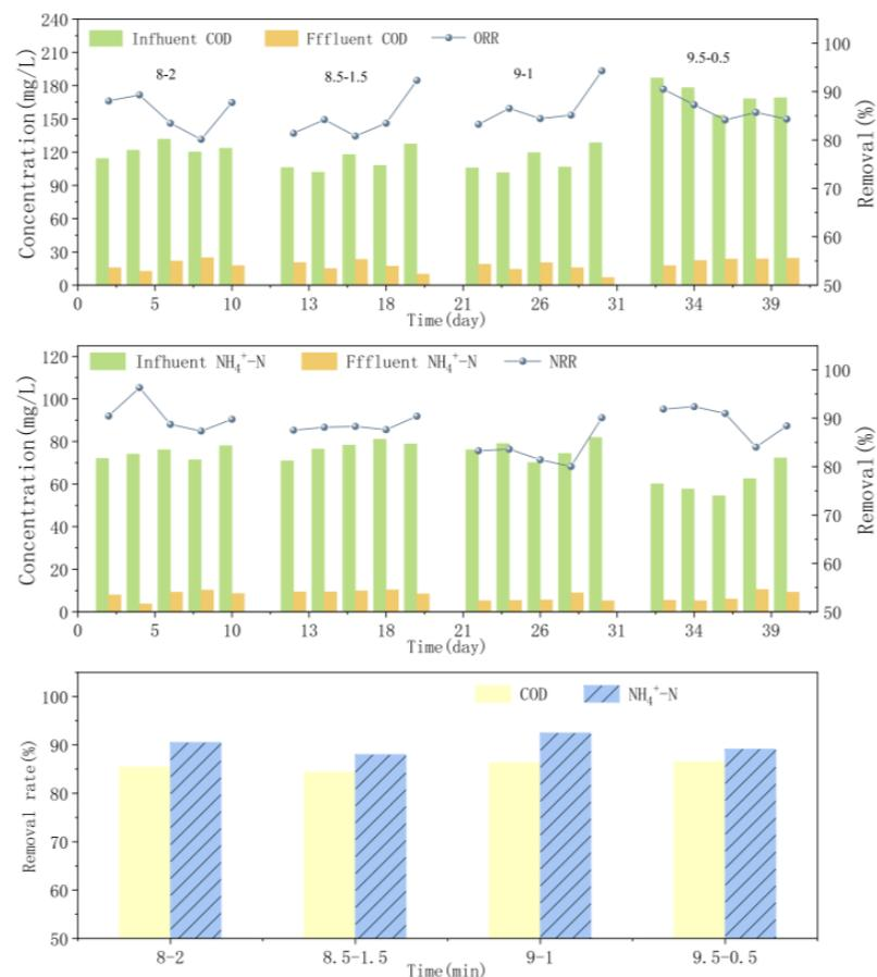
Figure 3. Removal of COD and  $\text{NH}_4^+\text{-N}$  under different filtration backwashing time.
