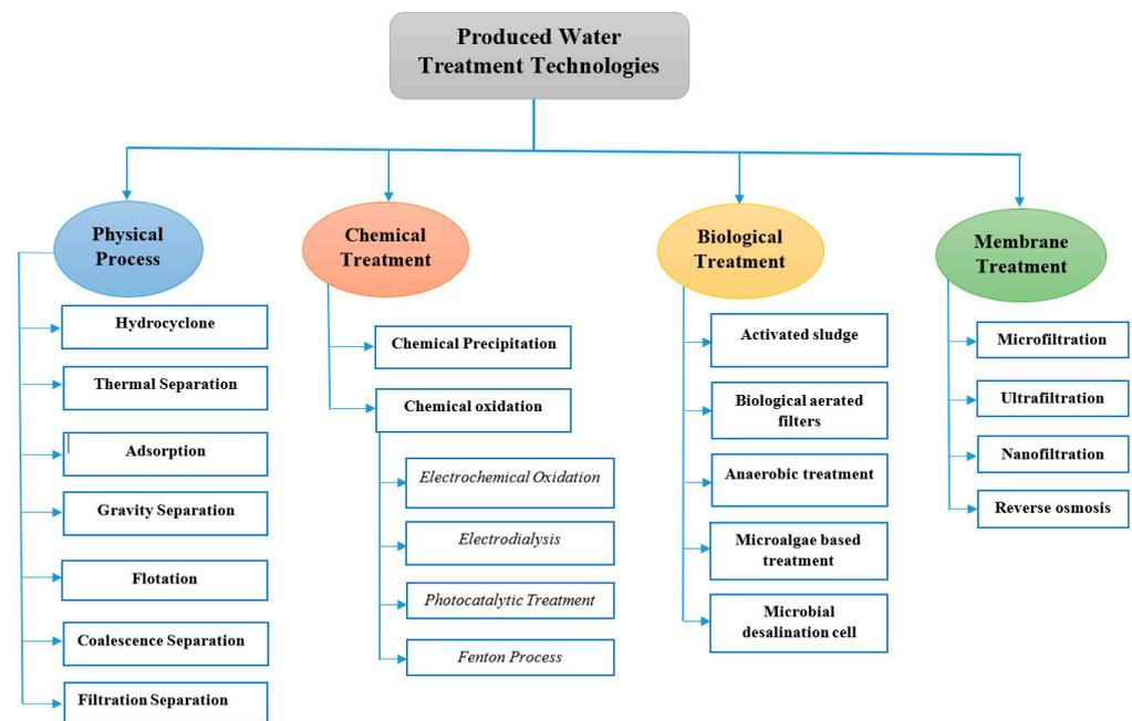
**Figure 12.** Flow chart for PW treatment technologies.
