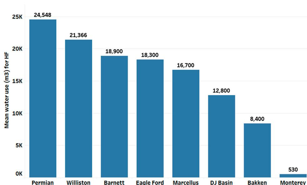
**Figure 8.** Average water use (m<sup>3</sup>) for HF (hydraulic fracturing) of horizontal wells in major shale plays in USA (data from [63,64]).
