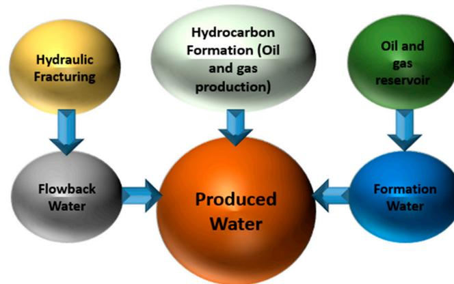
**Figure 2.** Different sources of produced water.
