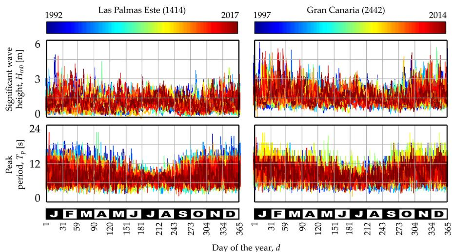
Figure 3. Measured values of significant wave height and peak period through the year.
