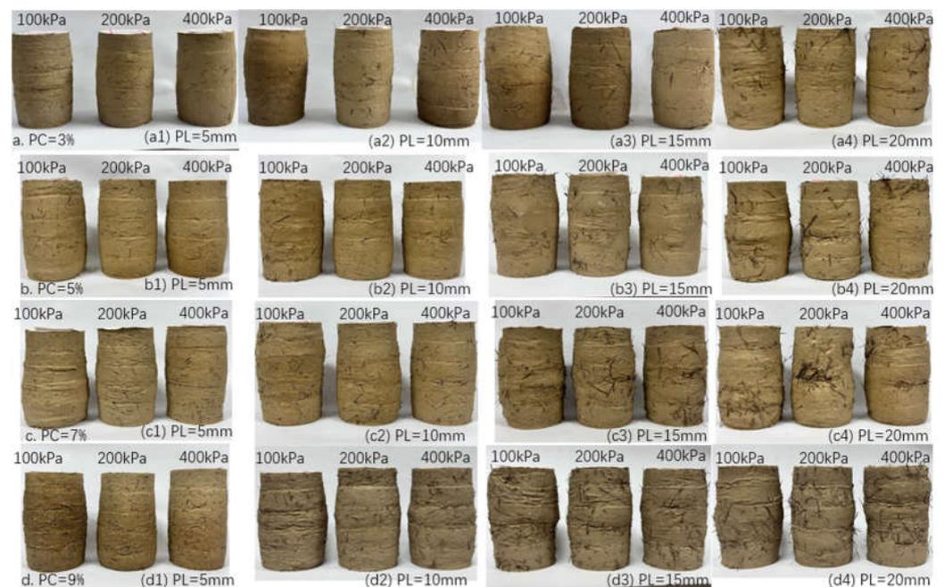
**Figure 7.** Failure samples for RTC condition with different fiber contents and fiber lengths: mass content in rows, (a) 0.3%, (b) 0.5%, (c) 0.7%, and (d) 0.9%; fiber length in columns, (1) 5 mm, (2) 10 mm, (3) 15 mm, (4) 20 mm.
