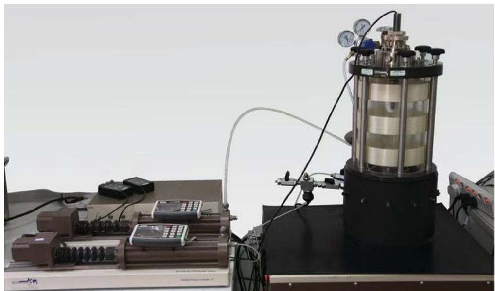
**Figure 3.** The triaxial apparatus from GDS located in the China Academy of Building Research.
