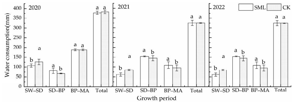
**Figure 6.** Water consumption in different growth periods. SW-SD indicates from the sowing to the seedling stage; SD-BP indicates from the seedling stage to the budding stage; and BP-MA indicates the budding to the maturity stage. Different lowercase letters above the bars indicate significant differences among the treatments at  $p < 0.05$ .
