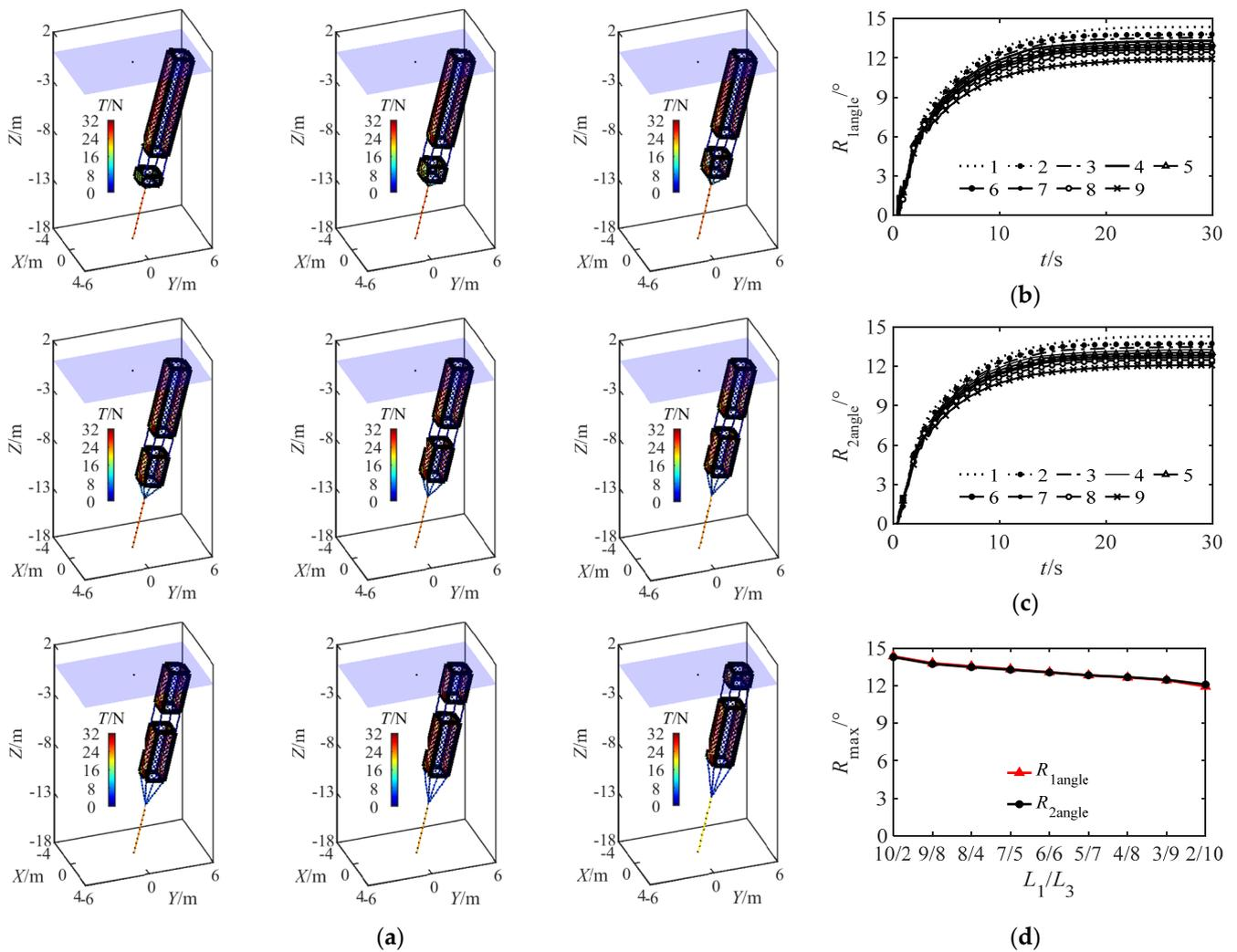
**Figure 4.** The effect of structural proportion of layered floating reef on reef movement. (a) Kinestate of the layered floating reef and force distribution of netting at the moment of maximum rolling angle; (b) time-varying of the upper reef rolling angle; (c) time-varying of the lower reef rolling angle; (d) effect of structural proportion on the maximum rolling angle of upper and lower reefs.
