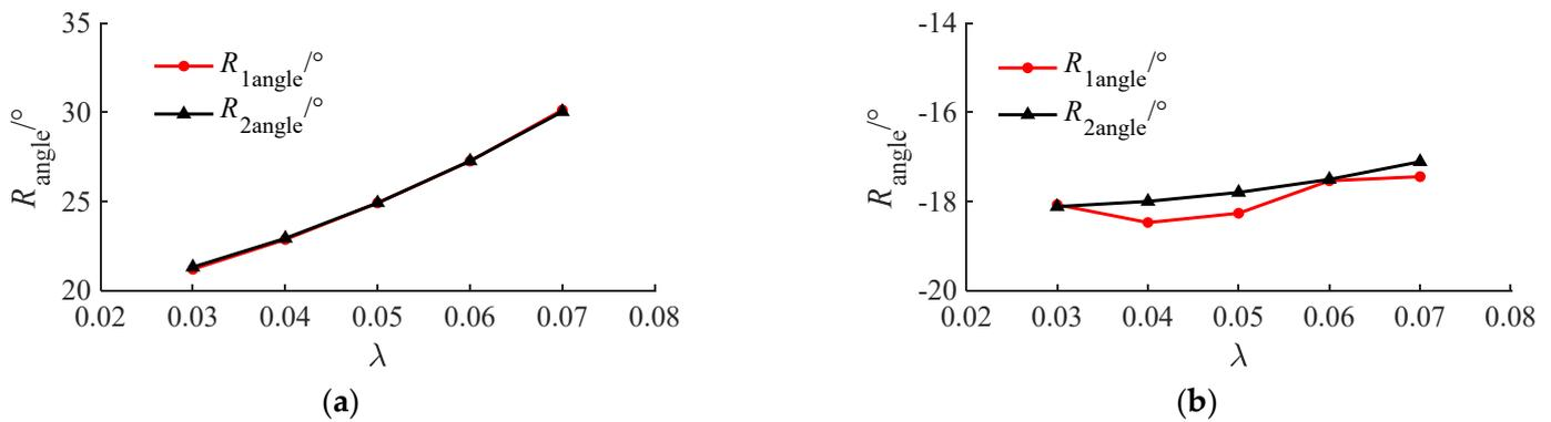
**Figure 8.** The maximum rolling angle of the reef varies with the wave steepness. (a) The maximum rolling angle of the upper and lower reefs varies with the wave steepness (downstream); (b) the maximum rolling angle of the upper and lower reefs varies with the wave steepness (upstream).
