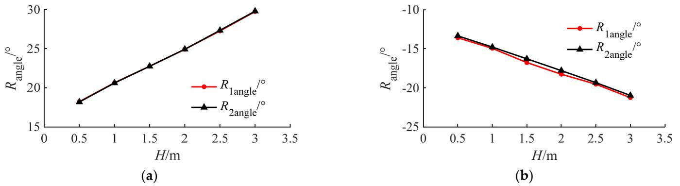
**Figure 6.** The maximum rolling angle of the reef varies with the wave height. (a) The maximum rolling angle of the upper and lower reefs varies with the wave height (downstream); (b) the maximum rolling angle of the upper and lower reefs varies with the wave height (upstream).
