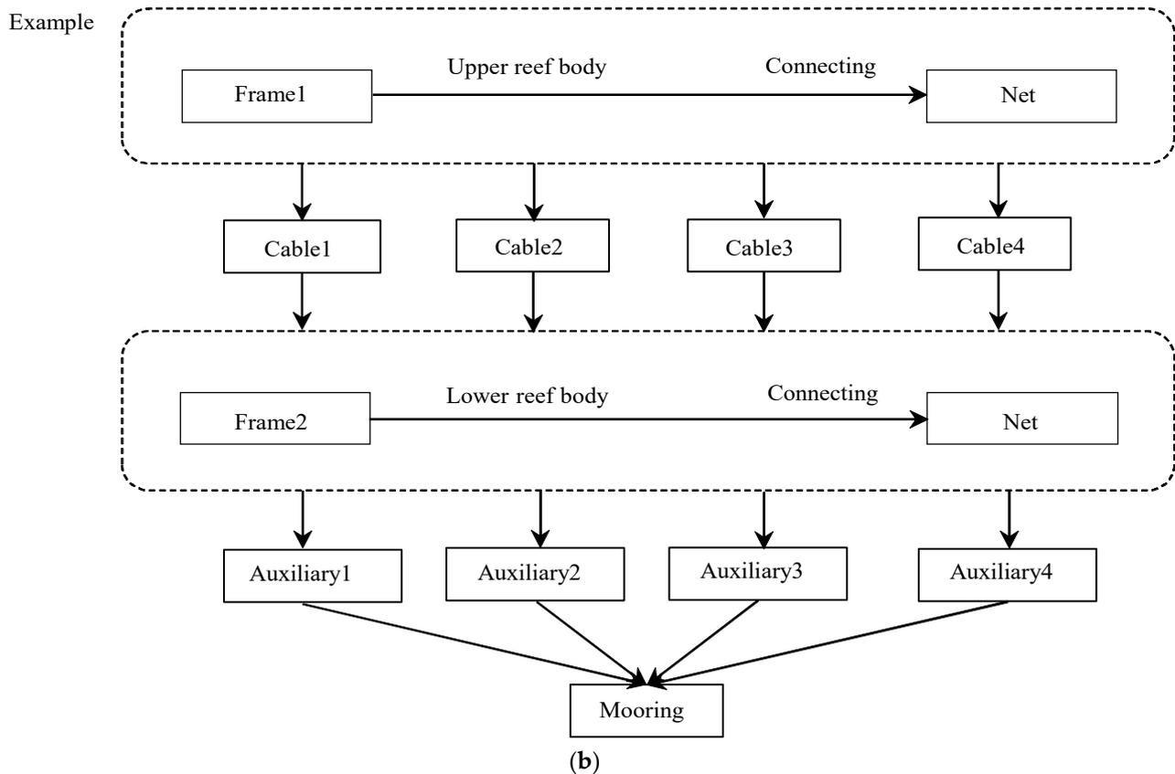
**Figure 2.** Program class library and example creation diagram of layered floating reef. (a) Layered floating reef class library diagram. (b) Layered floating reef example diagram.
