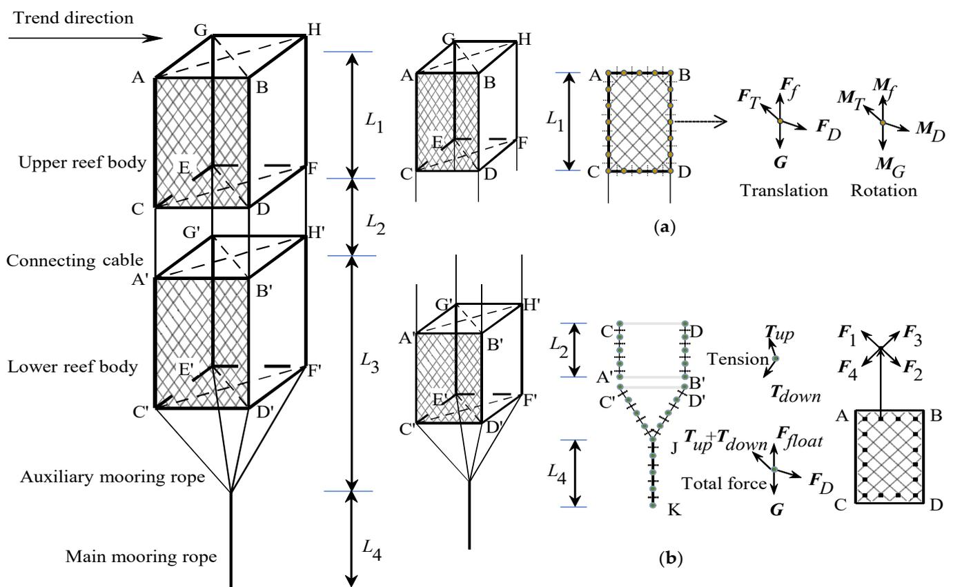
**Figure 1.** Structural diagram of layered floating reef. (a) Upper floating frame unit division and force diagram. (b) Lower floating reef unit division and force diagram.
