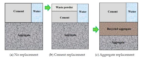
**Figure 2.** Schematic presentation of the use of alternative materials to replace the cement and aggregated in conventional cement mix design (copyrighted [47]).
