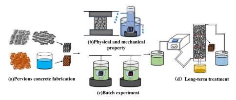
**Figure 10.** Experimental testing scheme for potential application of permeable materials in pollutant removal: (a) preparation of the monolith sample; (b) physical and mechanical characterizations; (c) static removal test; (d) dynamic removal test (copyrighted from [30]).
