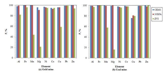
**Figure 12.** Removal performance of the different metals in the acid mine drainage from (a) gold and (b) coal mines (source data extracted from [176]).
