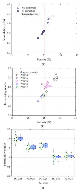
**Figure 9.** Effects of the mix design on the hydraulic properties of the hardened permeable concrete of different water to cement ration PC-X (X = 0.24; 0.26; 0.28; 0.3; 0.32): (a) effect of the incorporation of the admixture; (b) effect of the w/c ratio; (c) statistical distribution of the permeability at different w/c ratios (copyrighted from [123]).
