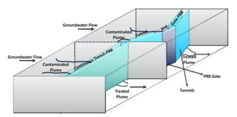
Figure 11. Configuration of the PRB designs: (copyrighted from [161]).
