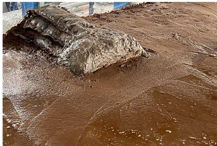
**Figure 7.** Mixed clay–geotube groin model (model dimensions: length 60 cm, width 45 cm, height 15 cm; the geotube part: 47 cm long, 45 cm wide, and 15 cm high; the clay part: 13 cm long, 45 cm wide, and 15 cm high).
