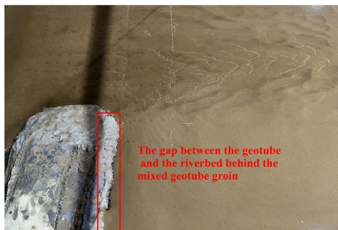
**Figure 21.** Partial diagram of the contact between the geotube behind the mixed clay–geotube groin and the riverbed.
