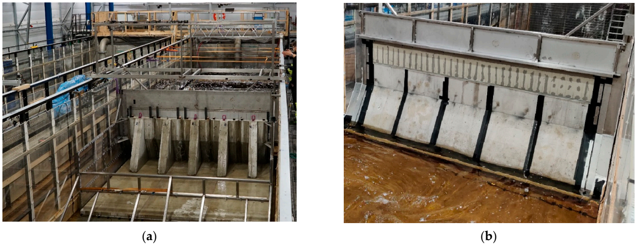
Figure 3. Photographs of the chute and the model showing (a) the downstream and (b) the upstream views. The rubber sheets used to seal the model are visible in image (b).
