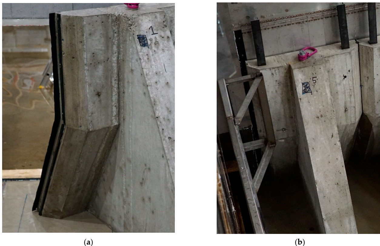
Figure 4. Details of the model: (a) the shear keys and (b) the side supports behind the outer monoliths.
