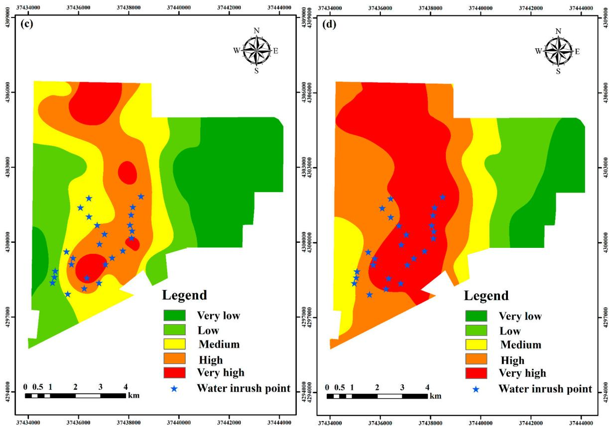
Figure 11. Verification diagram of the roof water inrush risk evaluation results under different risk-coping attitudes: (a)  $a = 0.1$ ; (b)  $a = 0.5$ ; (c)  $a = 0.7$ ; (d)  $a = 0.9$ .
