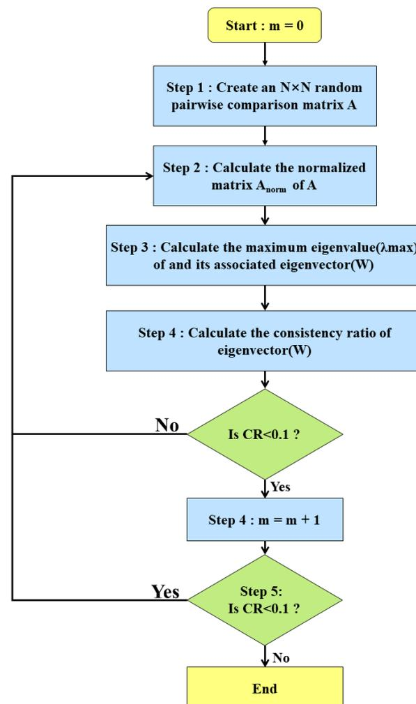
**Figure 4.** Flowchart for calculating the weights of the evaluation criteria by the Monte Carlo analytical hierarchy process.
