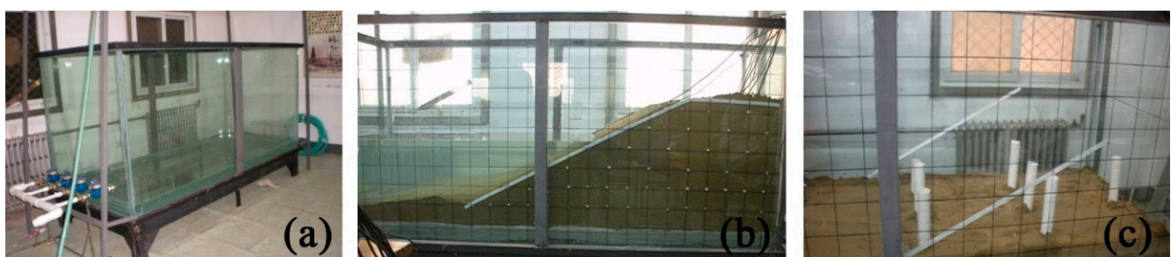
Figure 2. The layout of the model box and marking points: (a) model box; (b) mark point arrangement; (c) instrument burial.
