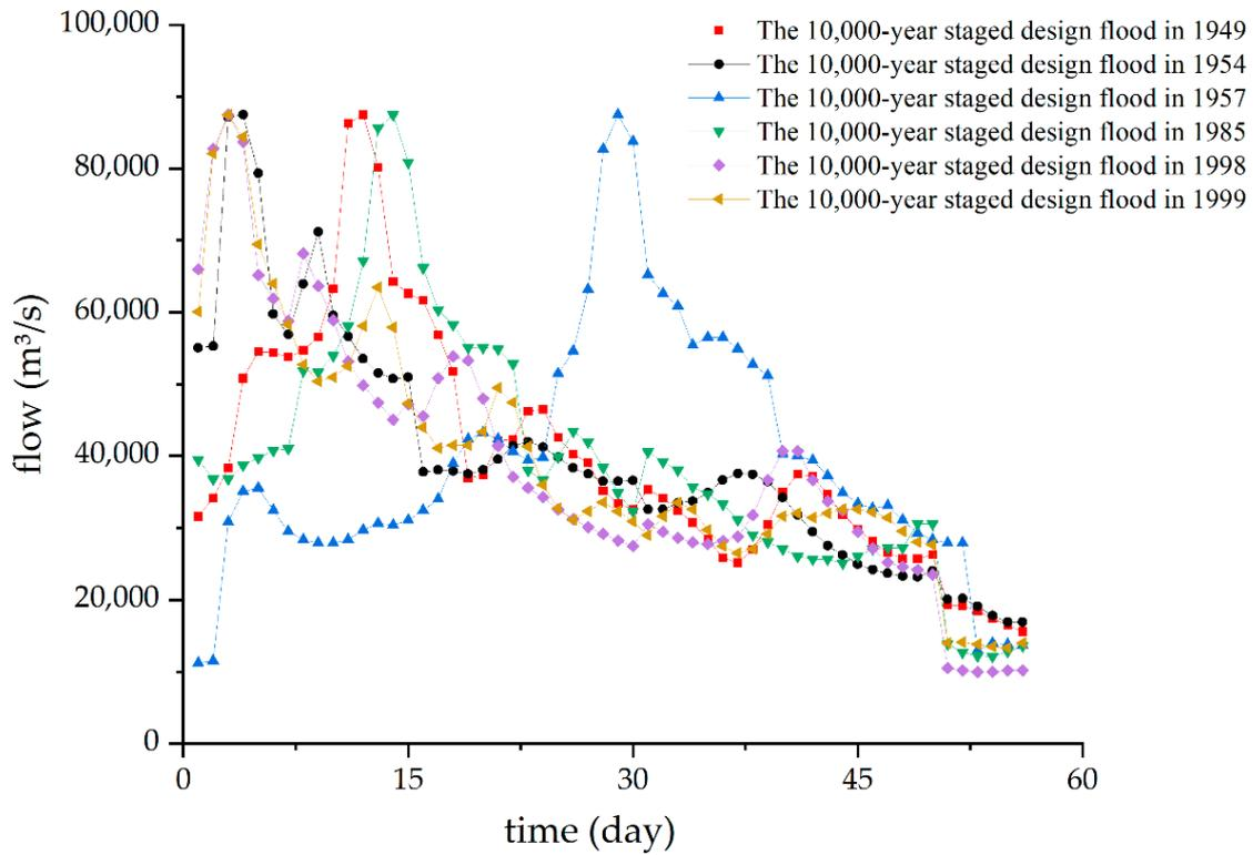
Figure 3. The 0.01% staged design floods for the Three Gorges Reservoir.
