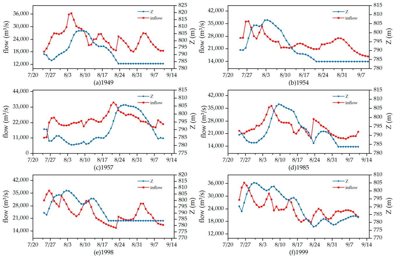
Figure 6. Flood risk analysis chart for the Baihetan Reservoir.
