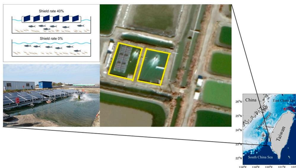
**Figure 1.** Comparison of ponds for culturing *Litopenaeus vannamei* and *Chanos Chanos* with floating solar photovoltaic panels between a shading rate of 40% and a shading rate of 0% at 23°07'24.41" N 120°04'49.67" E (image taken from Google Maps).
