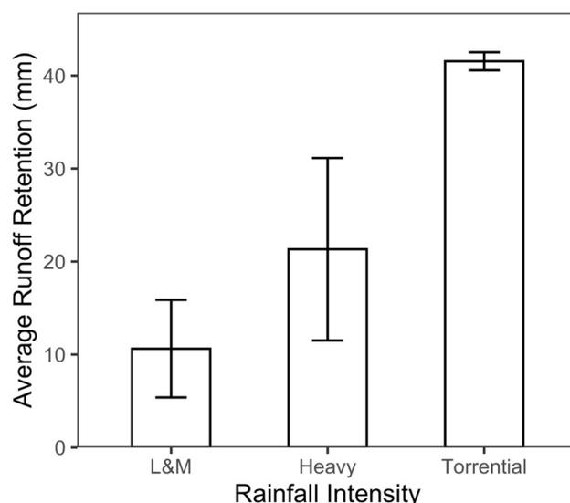
**Figure 4.** The average runoff retention of LID combination under three different rainfall intensity scenarios. The data in the bar plot represent the mean  $\pm$  standard deviation for each rainfall intensity scenario. Abbreviations: L&M—light and moderate rainfall.
