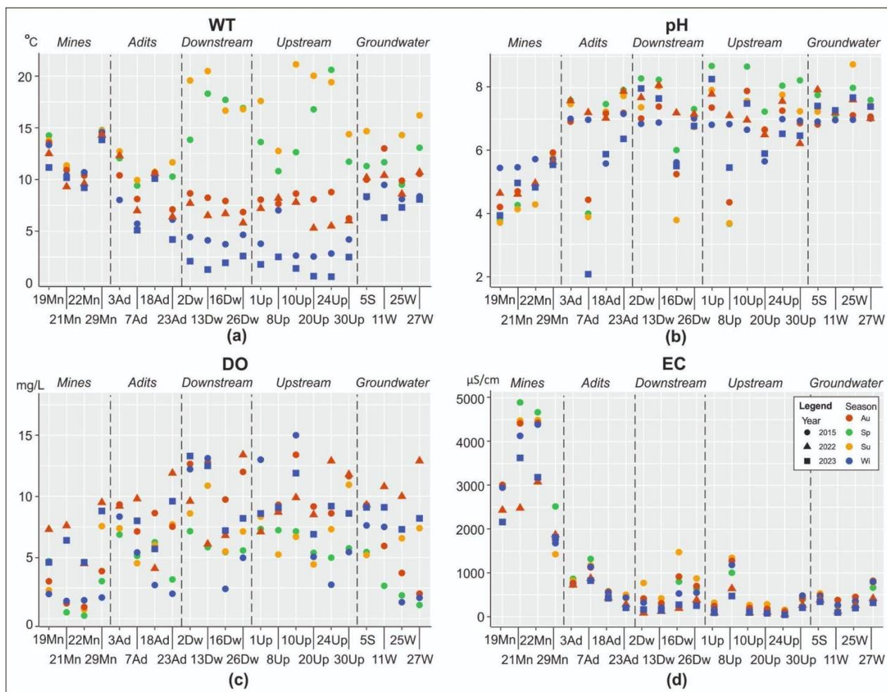
**Figure 2.** Individual value plots showing the seasonal and yearly distribution of the: (a) Water temperature (WT), (b) pH, (c) Dissolved Oxygen (DO), and (d) Electrical Conductivity (EC) of the 22 waters sampled in the GMAZ. The acronyms correspond to the sampled water sites (see Table 1).
