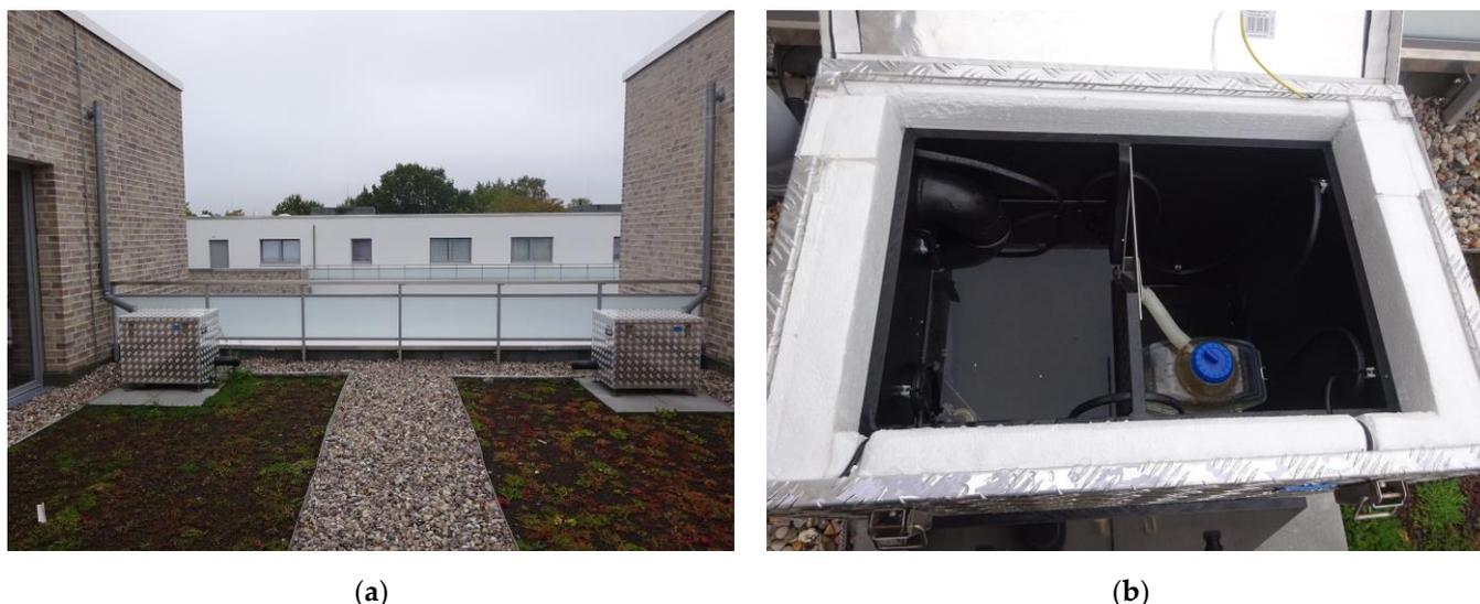
**Figure 4.** Photographs of the measurement boxes containing the tipping counters (a) and of the dual measurement (b) system with Thompson weir ((b) left side) and polycarbonate counter ((b) right side).
