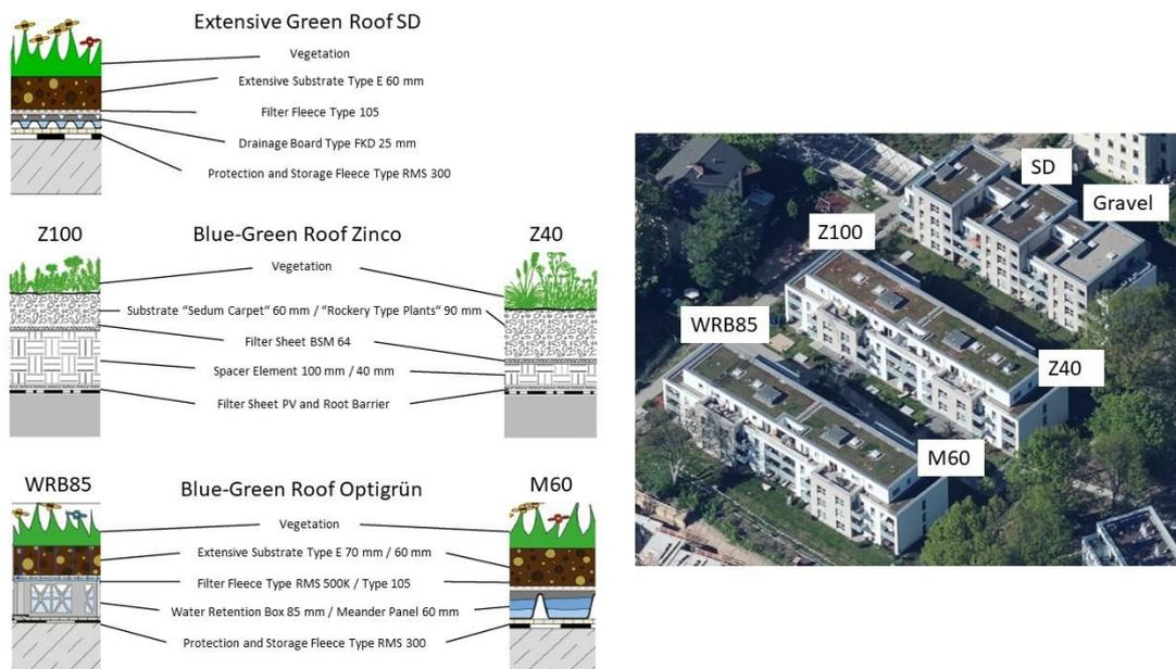
**Figure 3.** Diagrams of the different (B)GR systems, one extensive GR and four types of BGRs on two different buildings. In the 3D view of the residential buildings, the different roof types are marked. (GR system drawings provided by: Optigrün International AG, Krauchenwies-Göggingen, Germany and Zinco GmbH, Nürtingen, Germany; 3D view provided by: Hamburg State Office for Geoinformation and Surveying LGV).
