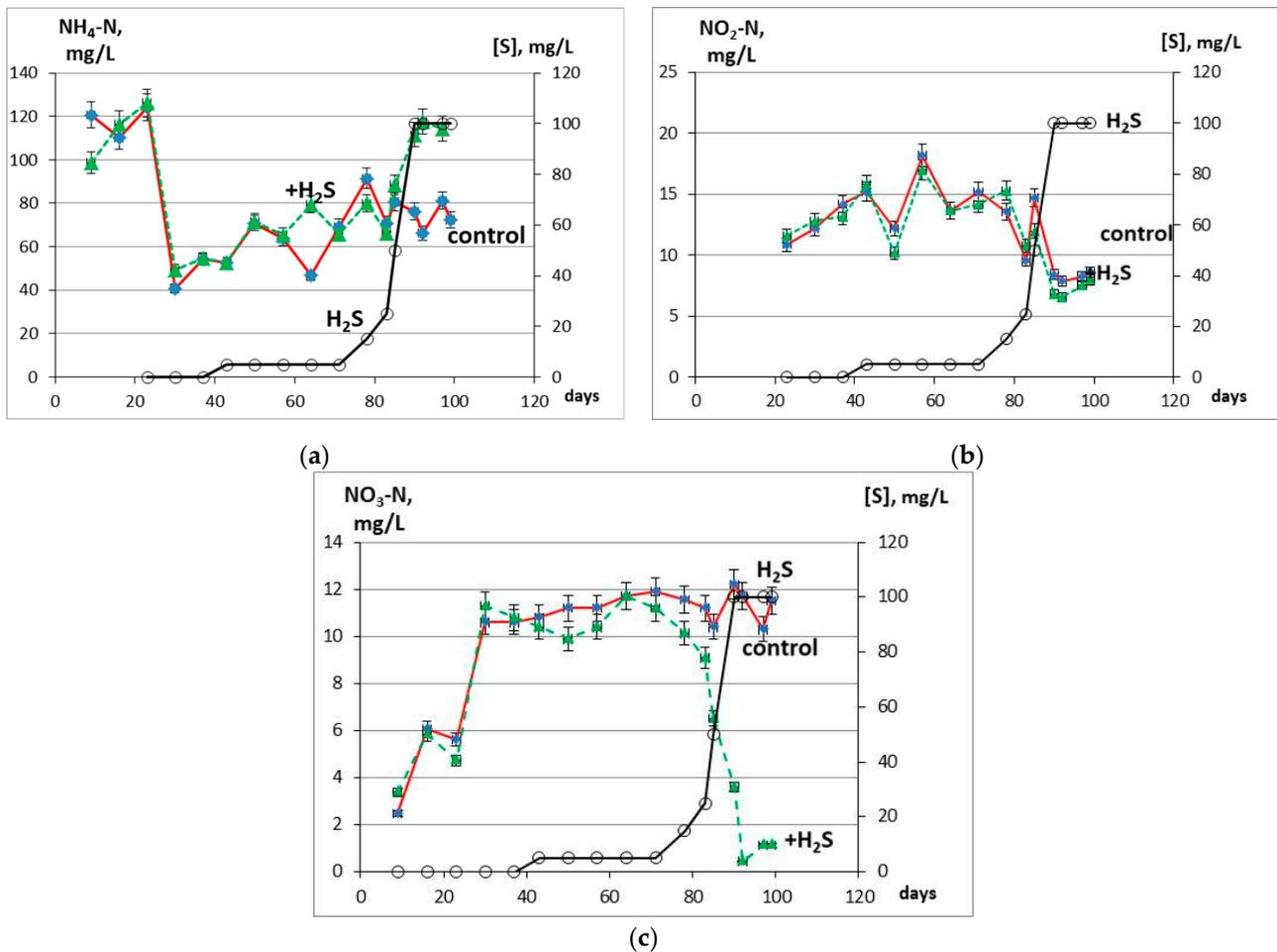
**Figure 2.** Dynamics of nitrogen species in the water treated in the anammox reactor: concentrations of ammonium (a), nitrite (b), and nitrate (c) in the control (red solid line) and experimental (green broken line) reactors. The black line shows sulfide concentration in the incoming water.
