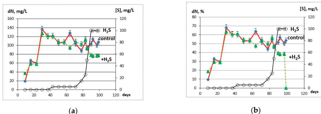
**Figure 1.** Operational parameters of the control (solid red line) and experimental (broken green line) bioreactors: nitrogen removal, dN, mg/L, (a) and its efficiency, % (b). The black broken line shows sulfide concentration in the incoming water.
