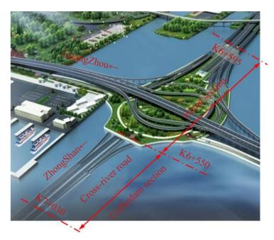
Figure 1. Plane position of the cofferdam.
