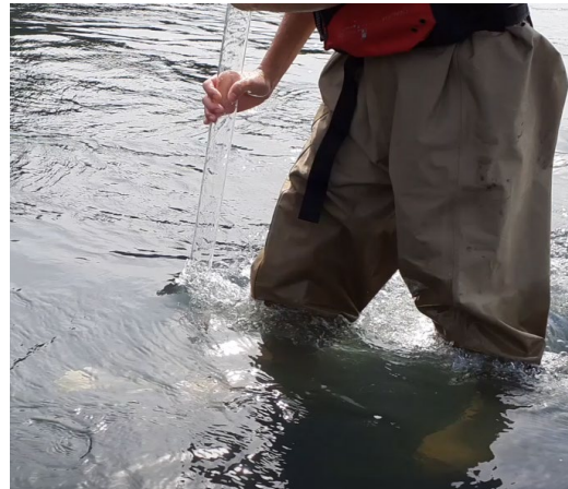
Figure 6. Measurement using a large pitot tube velocity meter.
