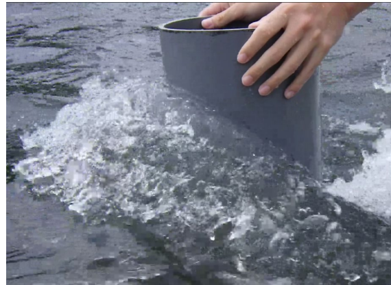
Figure 1. Observation of the afflux by the cylinder.
