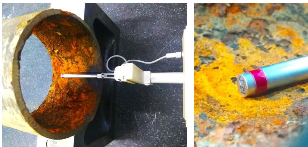
Figure 3. Measurement of roughness parameters with the Surtronic 3+ Taylor Hobson profilometer.
