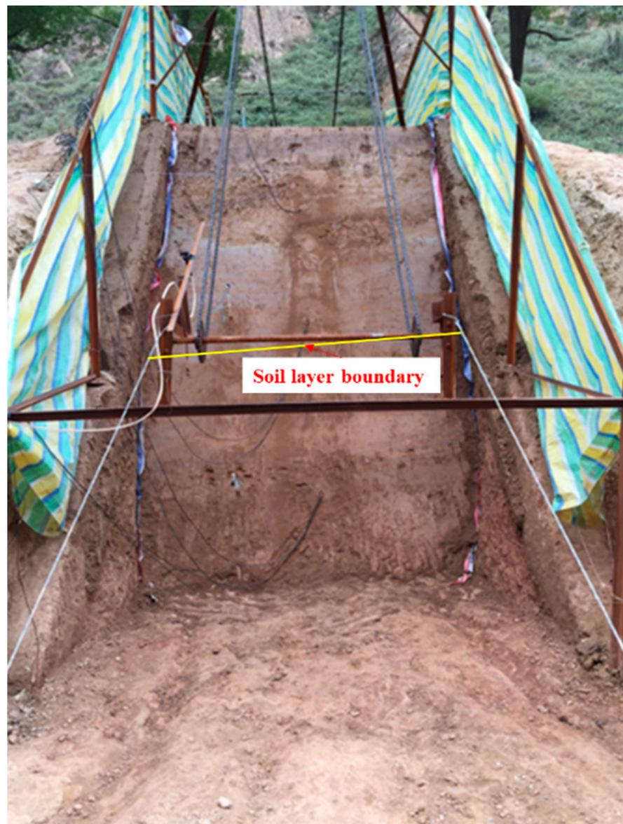
**Figure 1.** Schematic diagram of the test slope with slope cutting.
