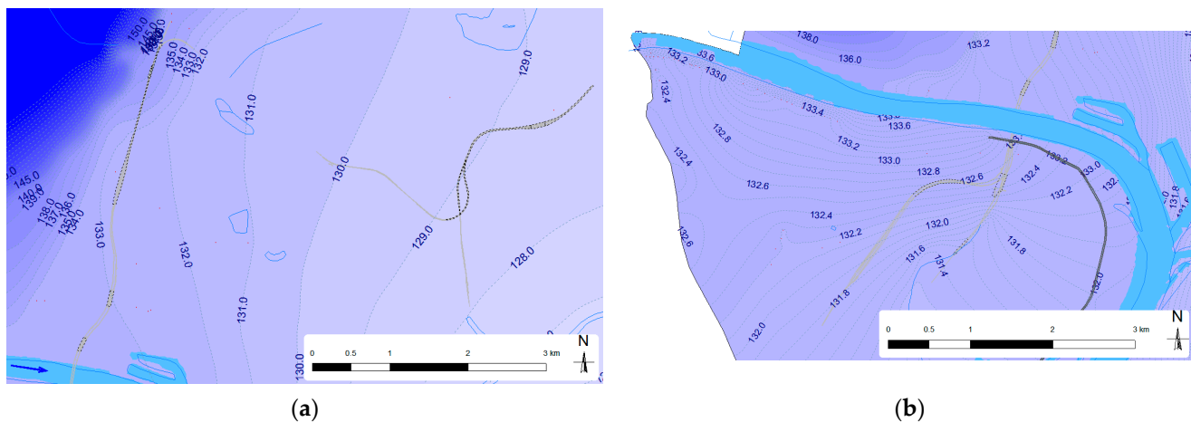
Figure 14. Course of simulated GWL isolines (m a.s.l.) for the maximum GWL state (for the month of April 2006): zoomed-in views of (a) the center of Bratislava and (b) the Petržalka region [17].
