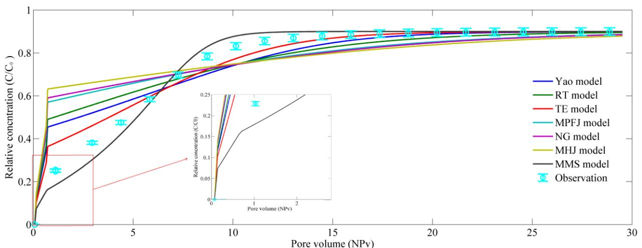
**Figure 5.** Comparison between the observed breakthrough curve (symbols) and simulated BTCs (solid line) with the existing models for the polydisperse particles, plotted as a function of the number of pore volumes (NPv). The mean concentration of five measurements, with the 95% confidence interval, is presented.
