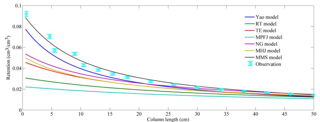
**Figure 7.** The comparison of the experimentally observed and simulated retention profiles for polydisperse particles along the sand column.
