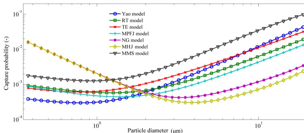
**Figure 4.** Comparison of the calculated capture probability for the polydisperse particles (0.375 to 18.863  $\mu\text{m}$ ) with the seven existing models. Data:  $\epsilon = 0.378$ ,  $u = 3.51 \times 10^{-5}$  m/s,  $\rho_p = 2.53 \times 10^3$  kg/m<sup>3</sup>,  $d_p = 2.932 \times 10^{-6}$  m,  $d_c = 5.03 \times 10^{-4}$  m,  $D = 2.31 \times 10^{-6}$  m<sup>2</sup>/s.
