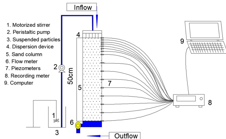
**Figure 2.** Illustration of the column experiment.
