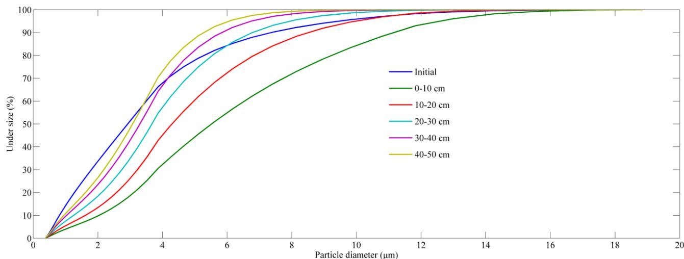
**Figure 10.** Particle size distribution (PSD) analysis of the retained polydisperse particles along the sand medium.
