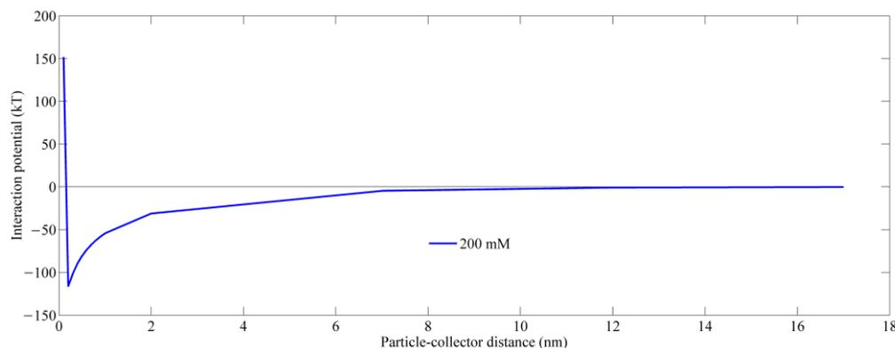
**Figure 3.** XDLVO energy profiles for the polydisperse particles and sand medium in 200 mM NaCl solution.
