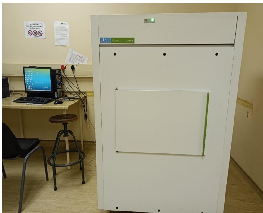
Figure 2. Perkin Elmer 1220 ultra-low-level liquid scintillation counter at the Center for Applied Radiation Science and Technology (CARST), North-West University (NWU), Mafikeng Campus, South Africa.
