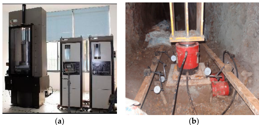
Figure 3. Laboratory and in situ tests. (a) Model MTS815-03 Triaxle Tester. (b) Original rock shear test.
