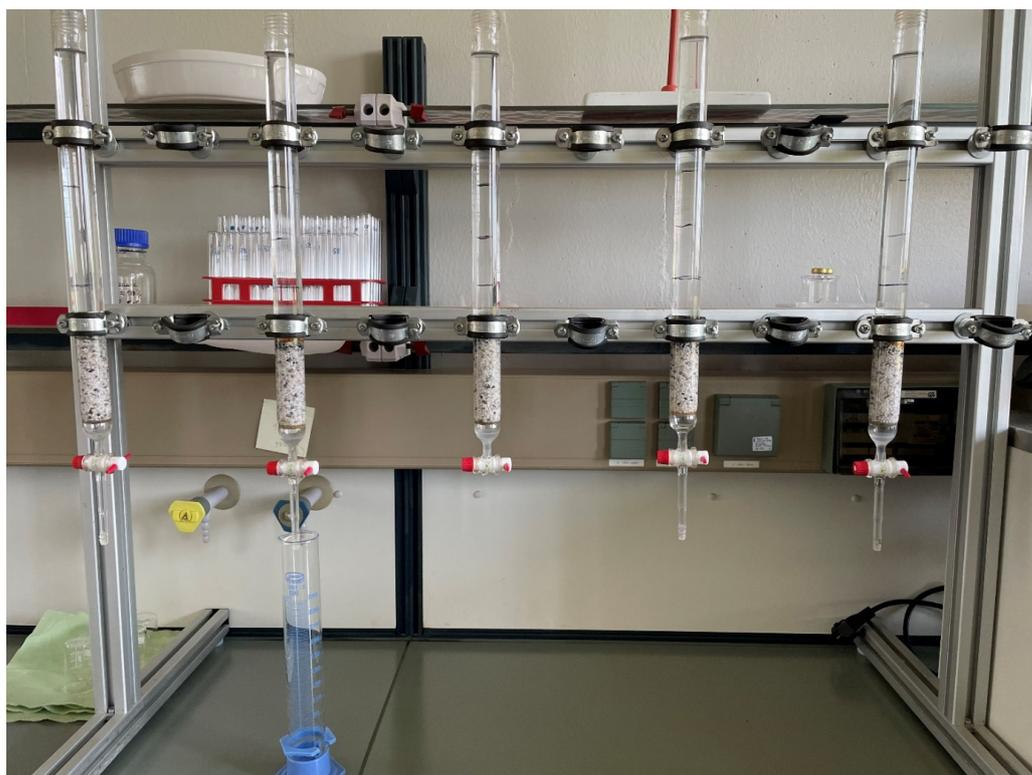
**Figure 1.** Column experimental set-up for  $\text{Fe}^0$  leaching by ascorbic acid (2 mM). The photograph was made at the end of the experiments. The spout of the third system was broken during the experiments but this has no incidence on the performance of the system.
