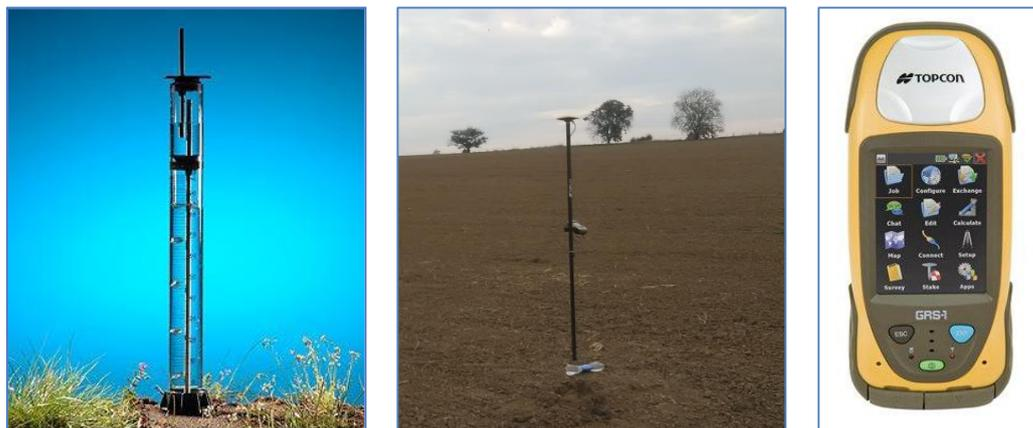
Figure 3. Mini disk infiltrometer and GPS Topcon device.
