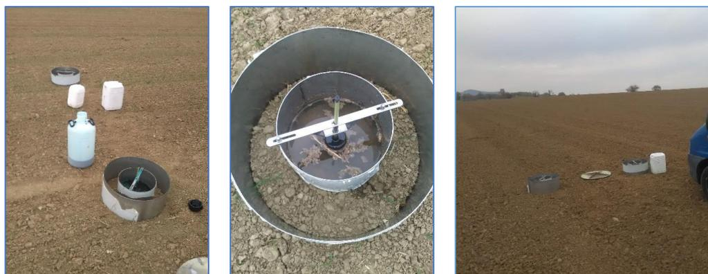
**Figure 4.** Double ring infiltrometer measurement.
