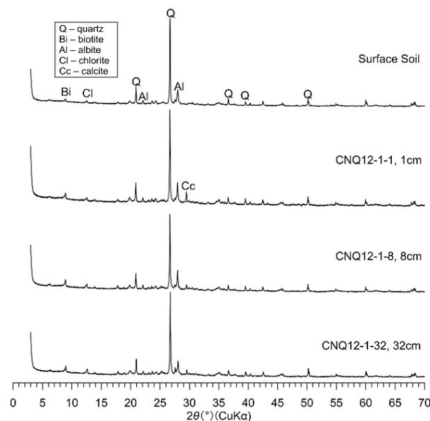
**Figure 4.** Results of XRD analysis for core CNQ12-1 and surface soils.
