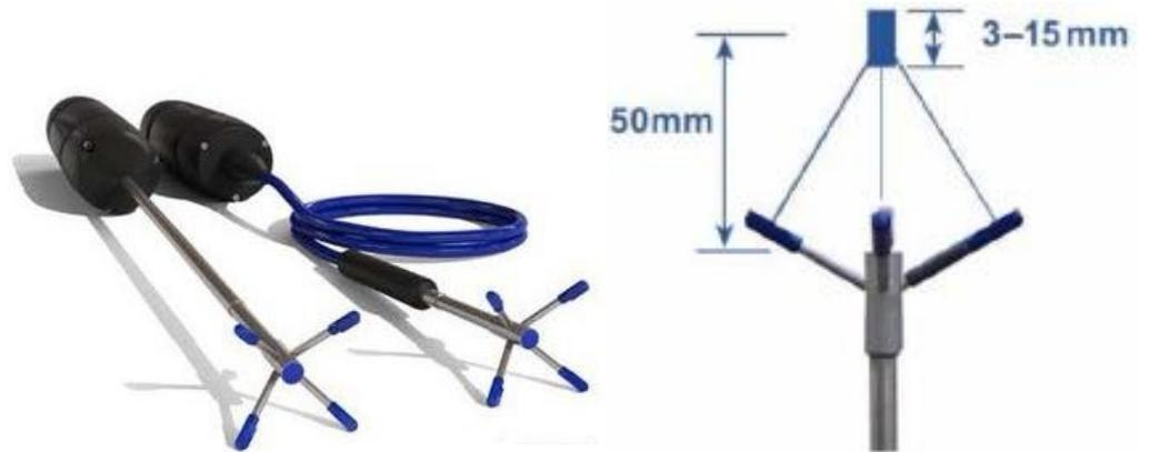
**Figure 6.** Acoustic Doppler Velocimetry (ADV).
