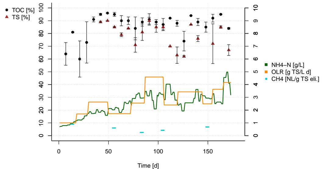
**Figure 4.** Mesophilic anaerobic digestion of slaughterhouse flotates at different organic loads.
