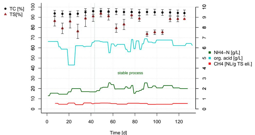
**Figure 9.** Thermophilic anaerobic digestion of slaughter waste mixed with wastewater at an organic load of  $4.2 \text{ g}_{\text{TS}} \cdot \text{L}^{-1} \cdot \text{d}^{-1}$ .
