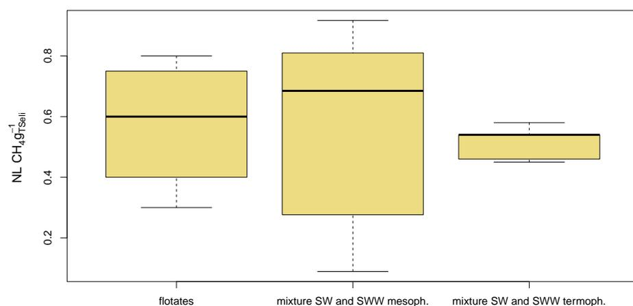
**Figure 11.** Comparison of the methane yields of the continuous experiments, without the first 40 days.
