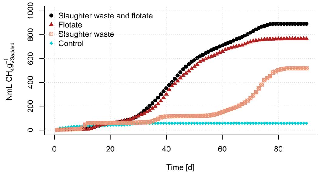
**Figure 3.** Trend of the methane yield for the biochemical methane potential measurements of the different substrates. The values represent the mean values of the three repetitions.
