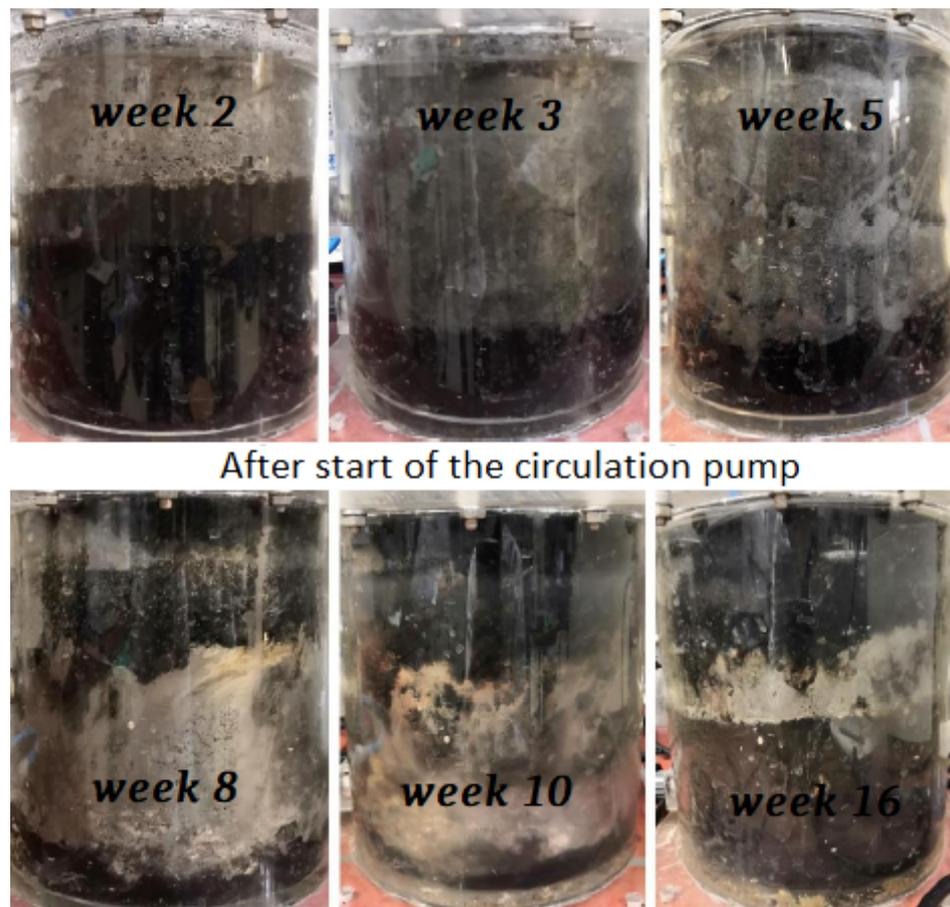
Figure 7. Grease layer built up in reactor over the experimental period with and without recirculation.
