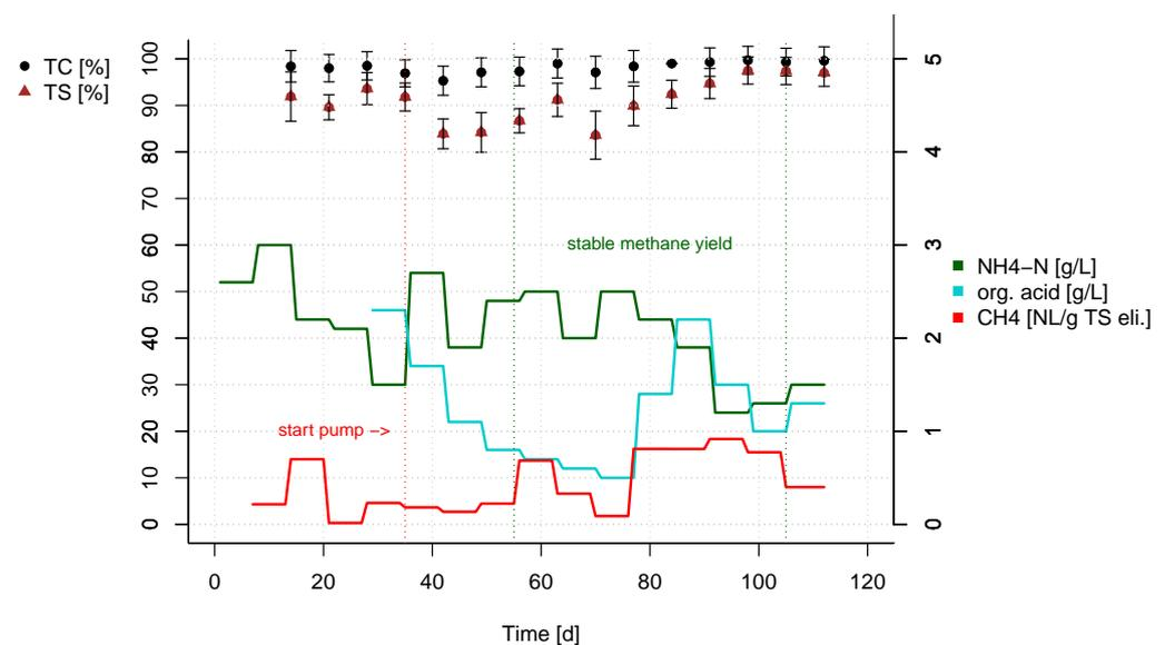
**Figure 6.** Mesophilic anaerobic digestion of slaughter waste and wastewater at an organic load of  $4.2 \text{ g}_{\text{TS}}\cdot\text{L}^{-1}\cdot\text{d}^{-1}$ .
