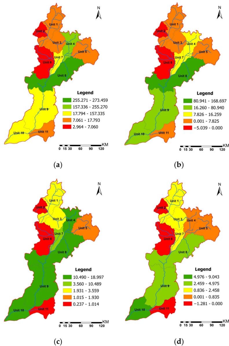
**Figure 5.** Spatial distribution of ideal and residual capacity of control units ((a): ideal capacity of NH<sub>3</sub>-N, (b): residual capacity of NH<sub>3</sub>-N; (c): Ideal capacity of TP, and (d): residual capacity of TP).
