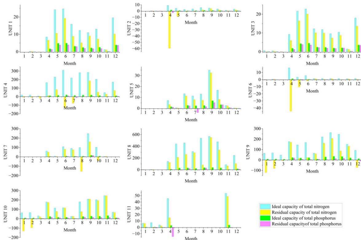
**Figure 6.** Monthly variation of water environment capacity in control units of Fenhe River Basin.
