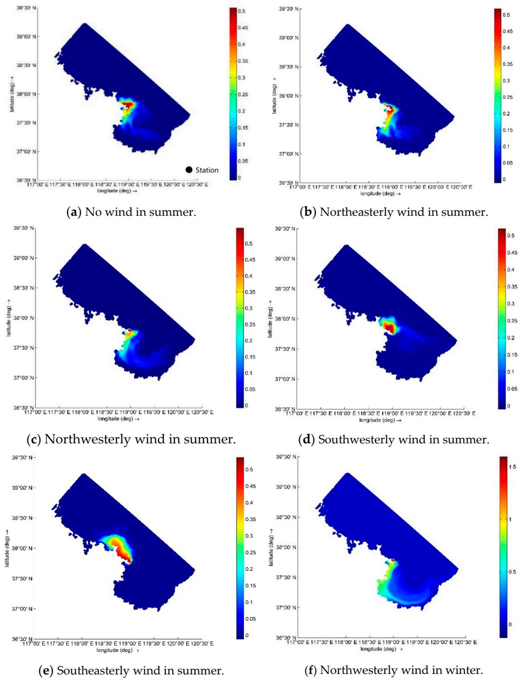
**Figure 7.** Suspended sediment transport at the Yellow River Delta under no wind (a), northeast wind (b), northwest wind (c), southwest wind (d), southeast wind (e) in summer and northwest wind (f) in winter (Unit: g/L) [30].
