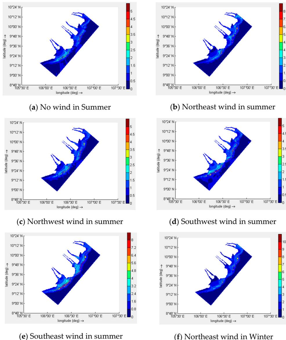
**Figure 4.** The shear stress on the bottom bed at the Mekong River Delta under no wind (a), northeast wind (b), northwest wind (c), southwest wind (d), southeast wind (e) in summer and northeast wind (f) in winter (Unit: Pa).
