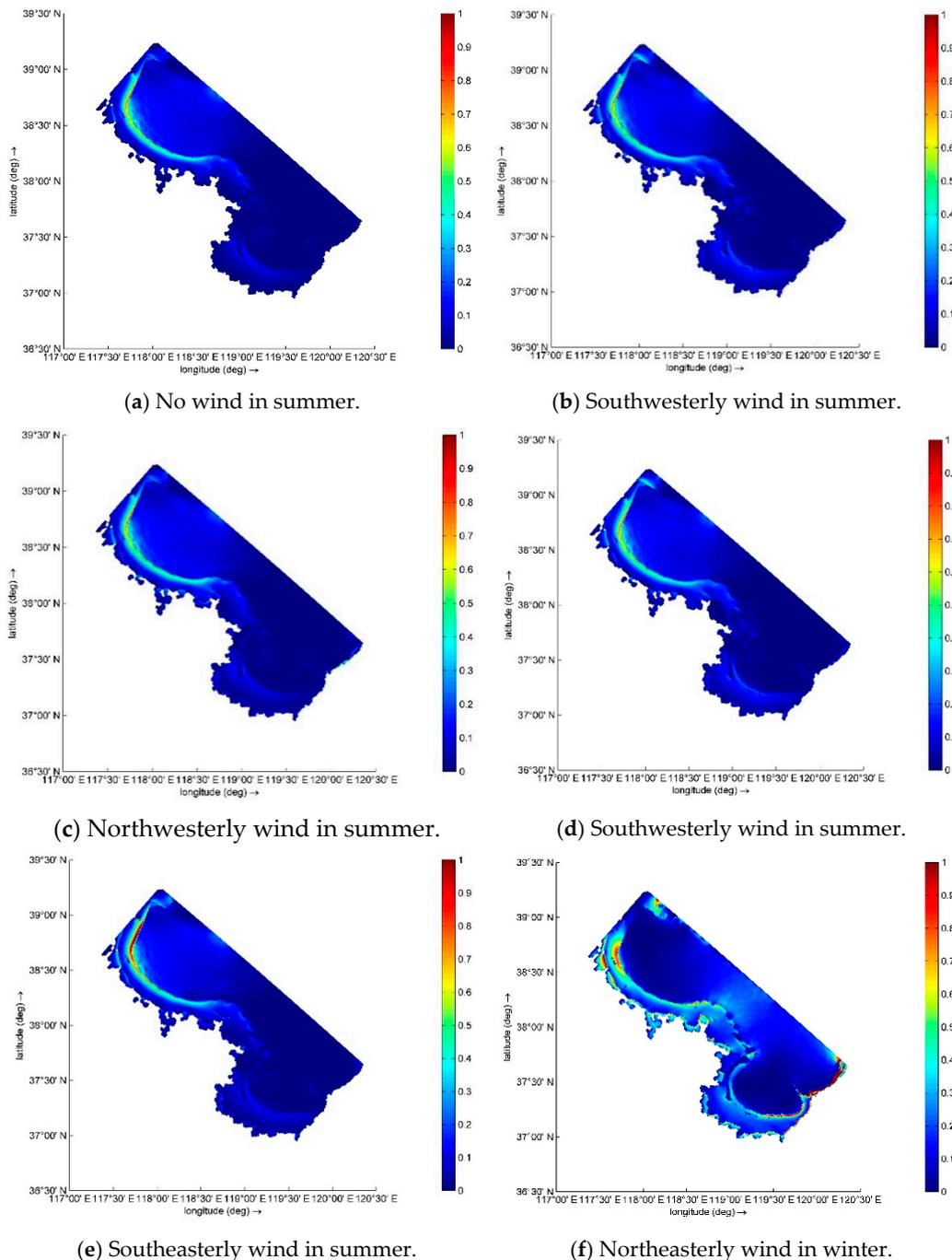
**Figure 5.** The shear stress on the bottom bed at the Yellow River Delta under no wind (a), northeast wind (b), northwest wind (c), southwest wind (d), southeast wind (e) in summer and northwest wind (f) in winter (Unit: Pa) [33].
