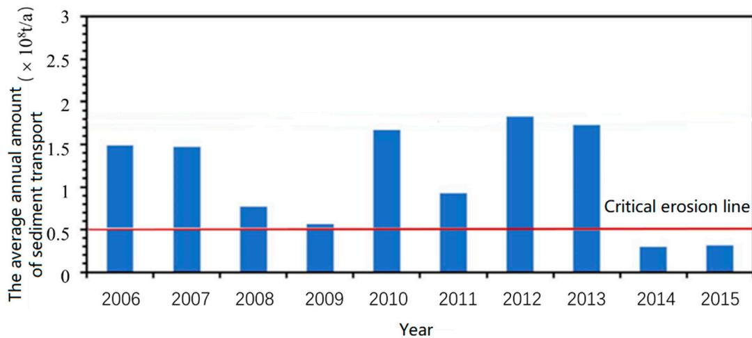
**Figure 10.** Annual erosion and deposition at the Yellow River’s subaqueous delta (data from the Yangtze River Sediment Bulletin).
