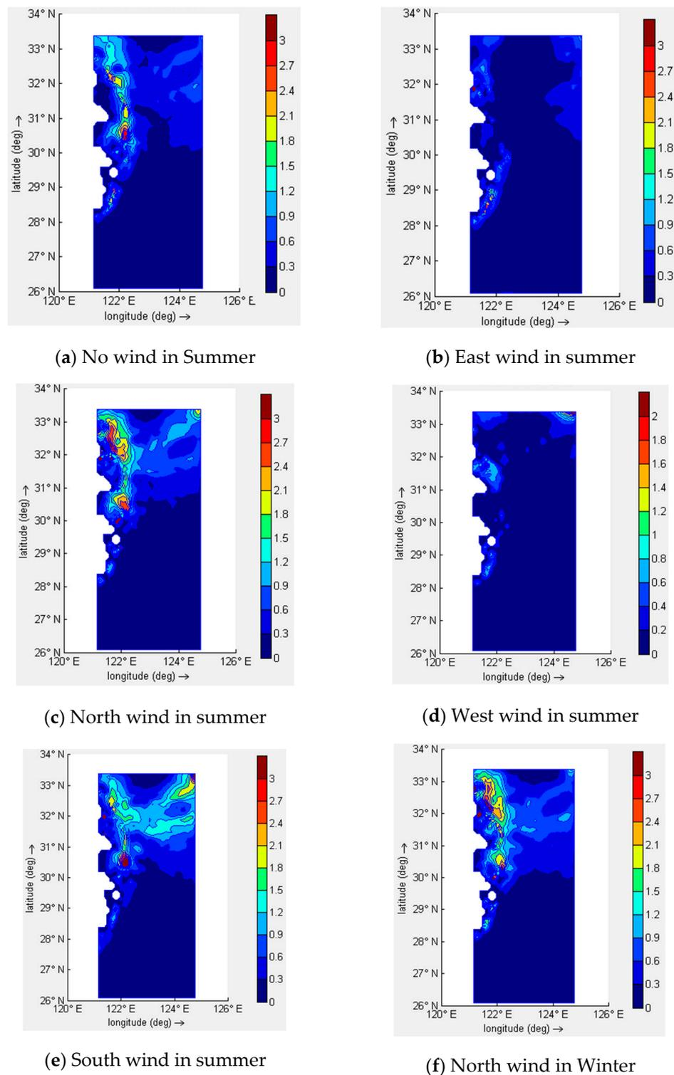
**Figure 9.** The shear stress on the bottom bed at the Yangtze River Delta under no wind (a), east wind (b), north wind (c), west wind (d), south wind (e) in summer and north wind (f) in winter (Unit: Pa) [30].
