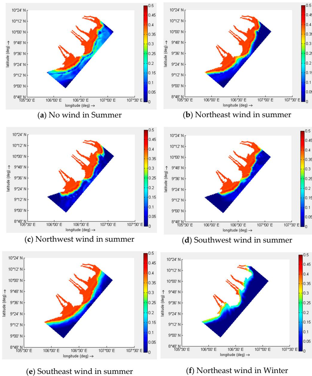
**Figure 3.** Suspended sediment transport at the Mekong River Delta under no wind (a), northeast wind (b), northwest wind (c), southwest wind (d), southeast wind (e) in summer and northeast wind (f) in winter (Unit: g/L).
