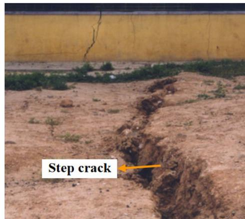
**Figure 3.** Surface step cracks in 6206 working face of Wangzhuang Coal Mine.
