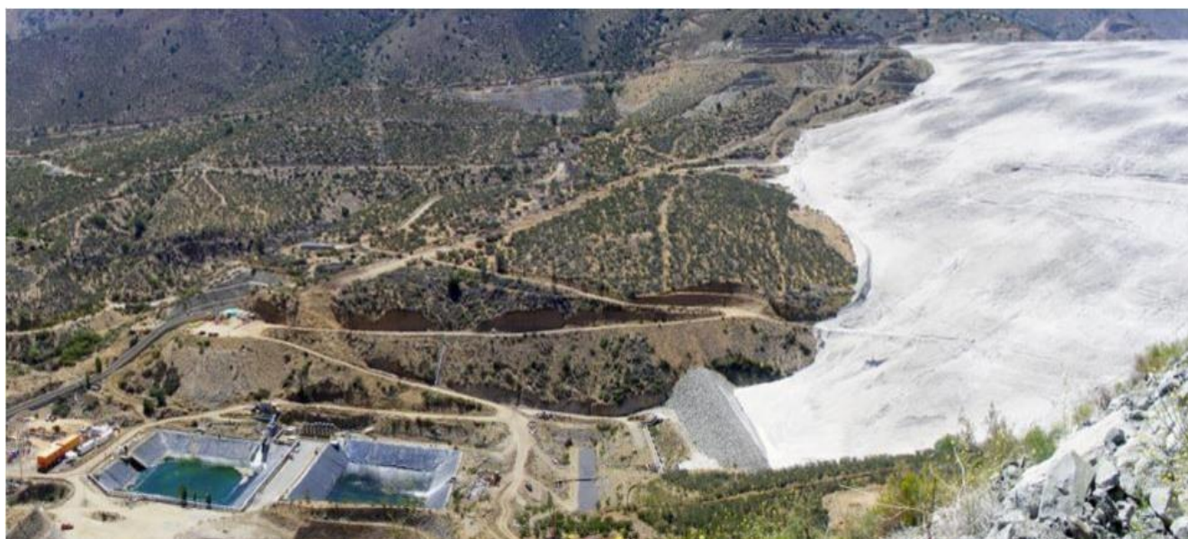
Figure 12. Seepage collection sumps in a TSF-Chile.
