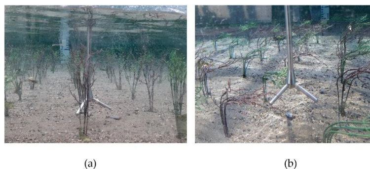
Figure 5. ADV position between two vegetation elements in (a) non-bending vegetation setting; (b) deflected vegetation setting.
