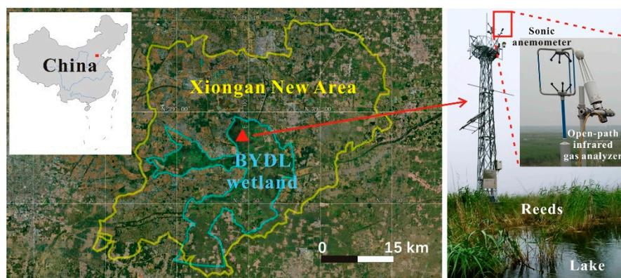
**Figure 1.** The location of the BYDL and the LI-COR 7500 eddy covariance analysis system for monitoring the meteorology and the wetland-air CO<sub>2</sub> exchange fluxes.
