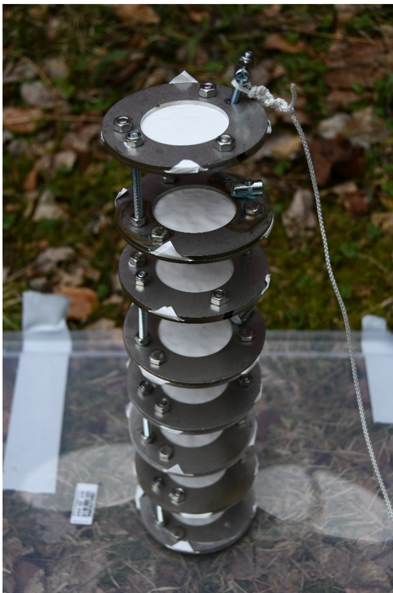
Figure S6. Photo of the POCIS prior to deployment into the groundwater well.
